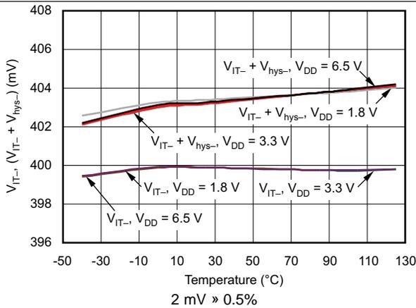
Figure 14. TPS386000-Q1 SENSE2 Threshold Voltage vs Temperature
