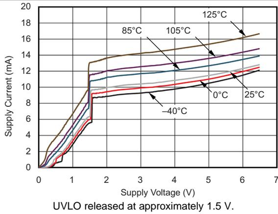
Figure 6. TPS386000-Q1 Supply Current vs Supply Voltage
