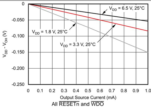
Figure 20. Output Voltage High vs Output Current
