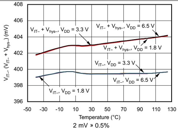
Figure 15. TPS386000-Q1 SENSE3 Threshold Voltage vs Temperature
