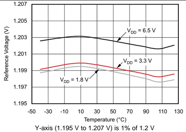
Figure 25. TPS386000-Q1  $V_{REF}$  at  $0\ \mu\text{A}$  vs Temperature
