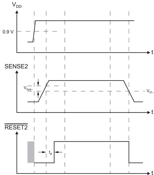
NOTE: The TPS386000-Q1 is shown here using  $\overline{\text{RESETn}}$ .
