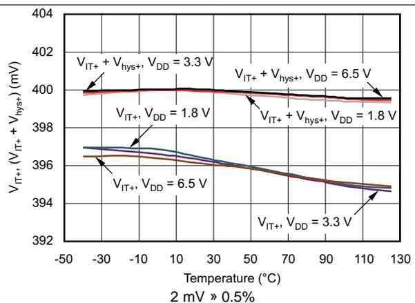
Figure 17. TPS386000-Q1 SENSE4H Threshold Voltage vs Temperature
