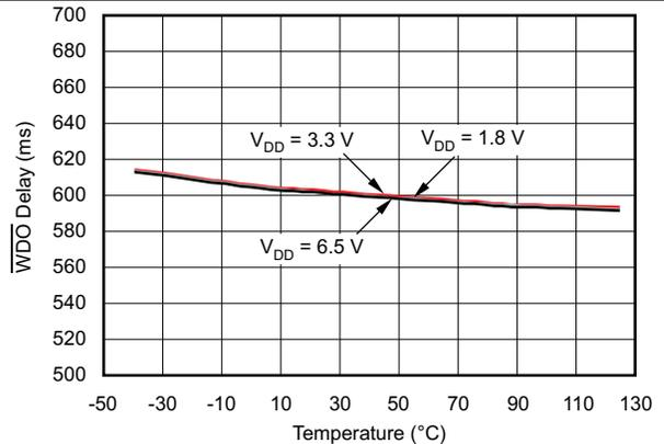
Figure 11. TPS386000-Q1 WDO Timeout Period vs Temperature
