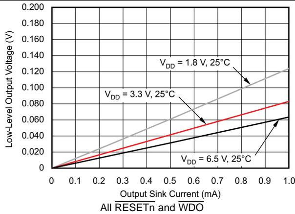
Figure 18. Output Voltage Low vs Output Current
