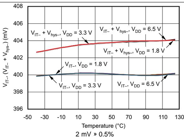
Figure 16. TPS386000-Q1 SENSE4L Threshold Voltage vs Temperature
