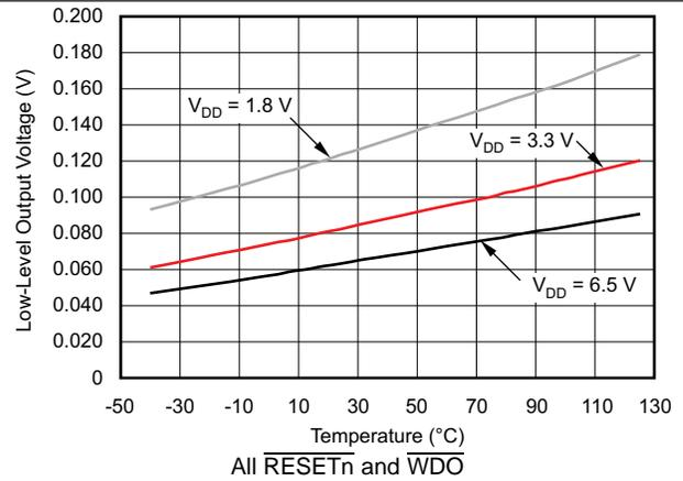
Figure 19. Output Voltage Low at 1 mA vs Temperature
