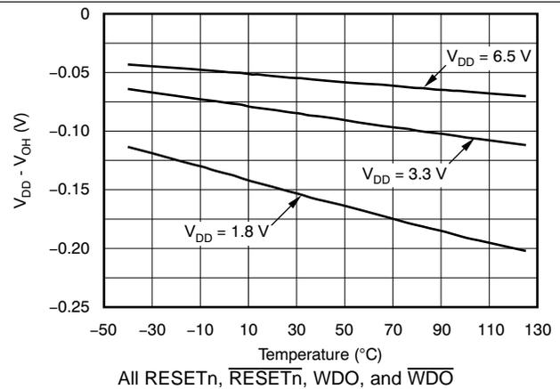
Figure 21. Output Voltage High at 1 mA vs Temperature
