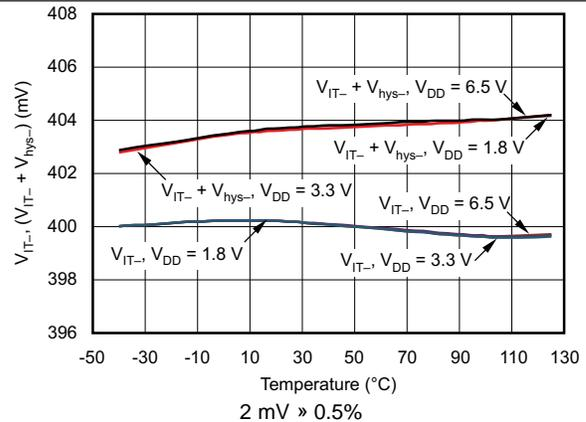
Figure 13. TPS386000-Q1 SENSE1 Threshold Voltage vs Temperature
