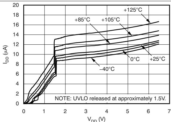
Figure 8. TPS386040 Supply Current vs Supply Voltage
