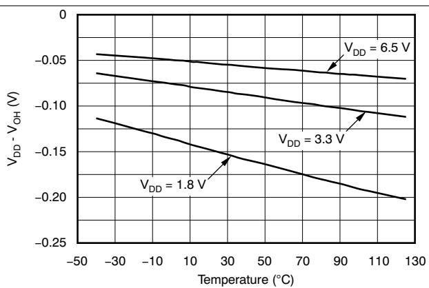
**Figure 23. Output Voltage High at 1 mA vs Temperature**
