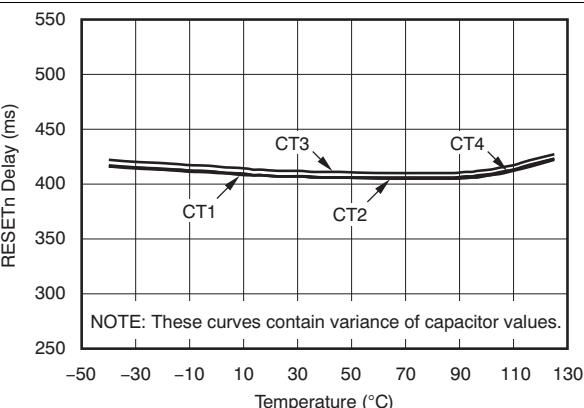
Figure 12. TPS386040 (CTn = 0.1  $\mu\text{F}$ )  $\overline{\text{RESET}_n}$  Time-out Period vs Temperature
