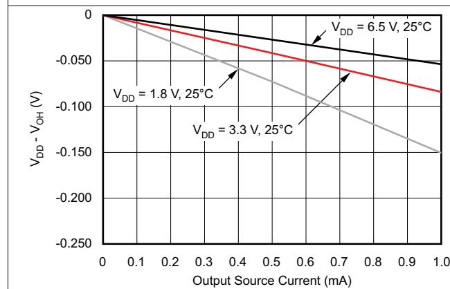
**Figure 22. Output Voltage High vs Output Current**
