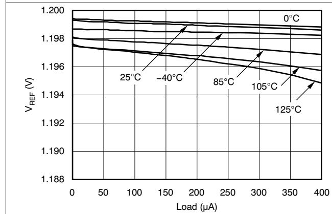
**Figure 24. TPS386040  $V_{REF}$  Output Load Regulation ( $V_{DD} = 1.8\text{ V}$ )**
