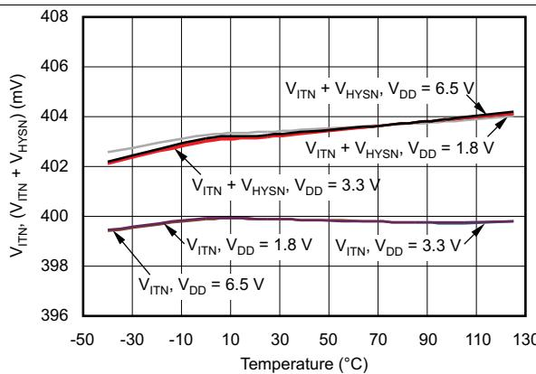
**Figure 16. TPS386040 SENSE2 Threshold Voltage vs Temperature**
