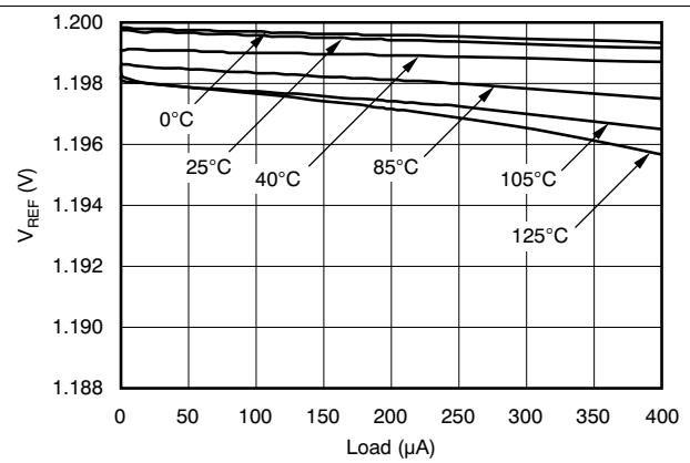
**Figure 25. TPS386040  $V_{REF}$  Output Load Regulation ( $V_{DD} = 3.3\text{ V}$ )**
