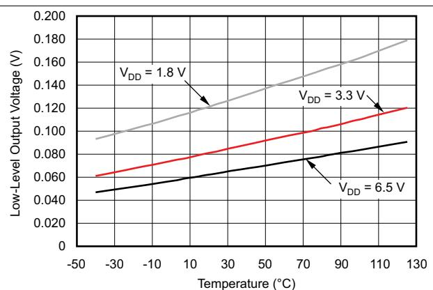
**Figure 21. Output Voltage Low at 1 mA vs Temperature**
