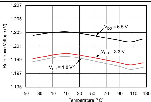
Figure 27. TPS386040  $\text{V}_\text{REF}$  at  $0\text{ }\mu\text{A}$  vs Temperature
