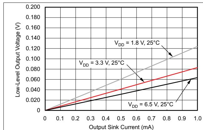
**Figure 20. Output Voltage Low vs Output Current**
