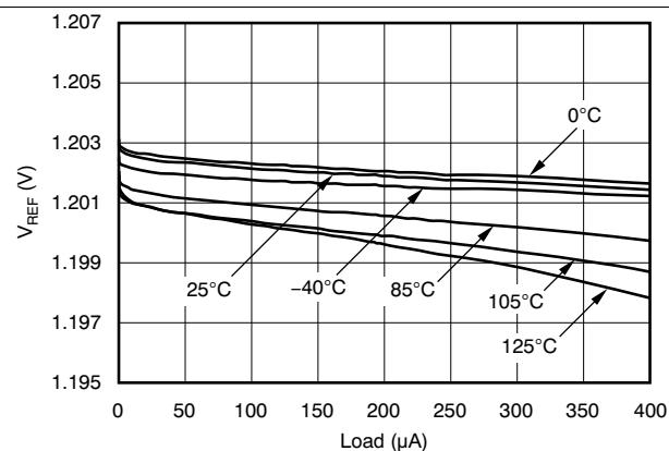
Figure 26. TPS386040  $\text{V}_\text{REF}$  Output Load Regulation
