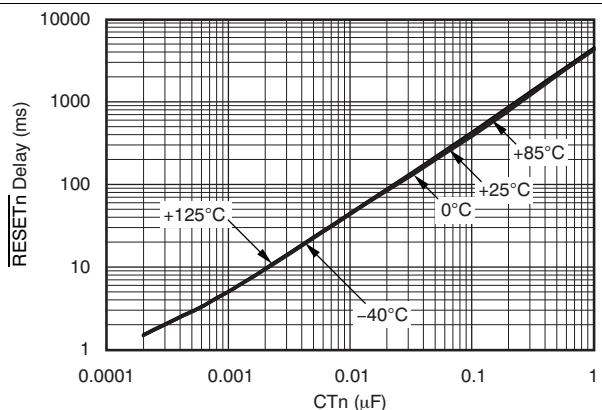
Figure 9. TPS386040  $\overline{\text{RESET}_n}$  Time-out Period vs  $CT_n$
