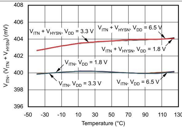
**Figure 18. TPS386040 SENSE4L Threshold Voltage vs Temperature**
