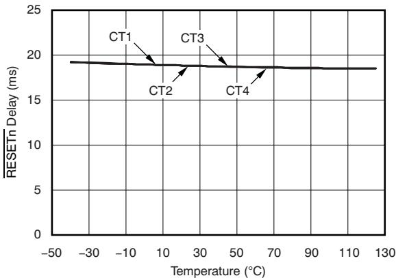
Figure 10. TPS386040 (CTn = Open)  $\overline{\text{RESET}_n}$  Time-out Period vs Temperature
