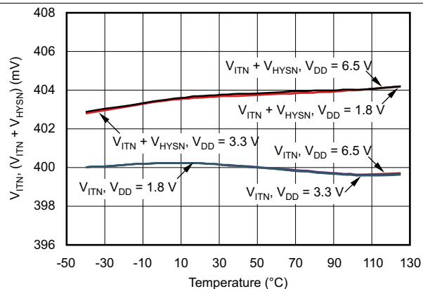
**Figure 15. TPS386040 SENSE1 Threshold Voltage vs Temperature**
