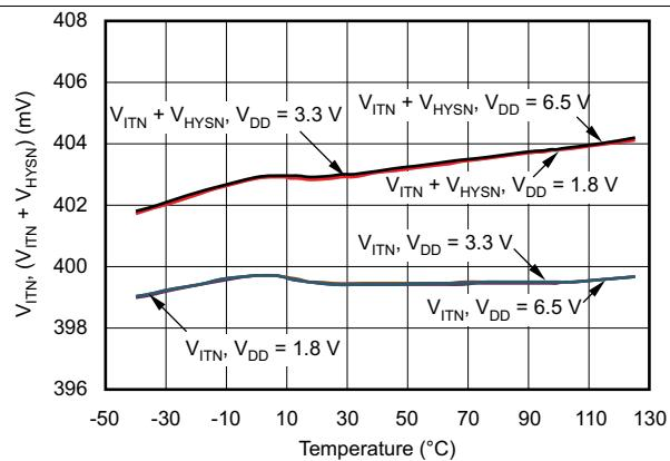
**Figure 17. TPS386040 SENSE3 Threshold Voltage vs Temperature**
