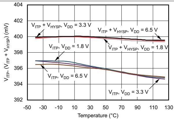
**Figure 19. TPS386040 SENSE4H Threshold Voltage vs Temperature**
