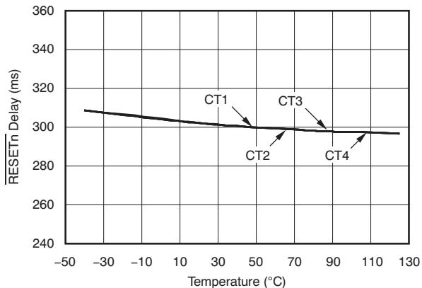
Figure 11. TPS386040 (CTn =  $V_{DD}$ )  $\overline{\text{RESET}_n}$  Time-out Period vs Temperature
