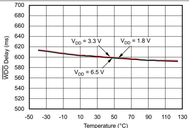
Figure 13. TPS386040  $\overline{WDO}$  Time-out Period vs Temperature
