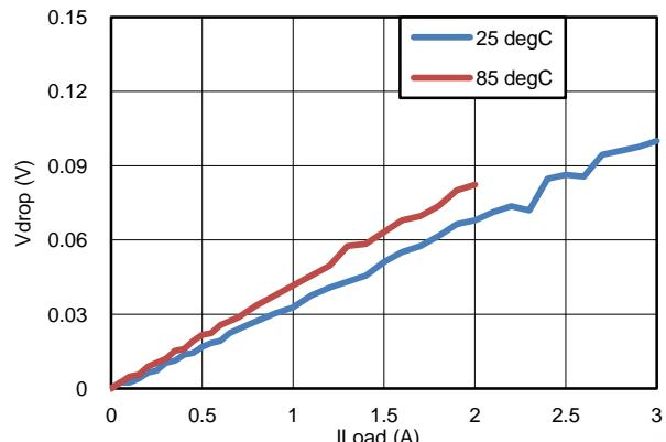
Figure 15. Vdrop vs IL;  $V_{GSQ1} = -5.5V$
