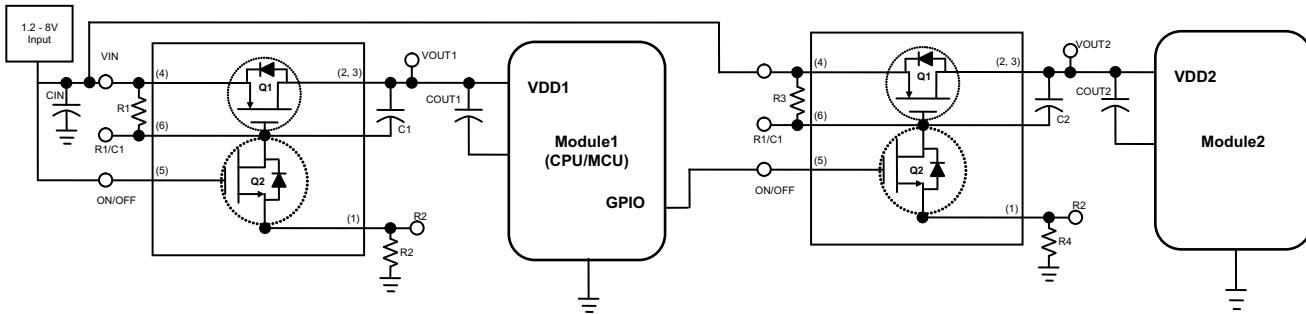
**Figure 8. Power Sequencing Using TPS27081A, Example 2**
