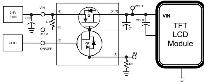
**Figure 4. Inrush Current Control Using TPS27081A**
