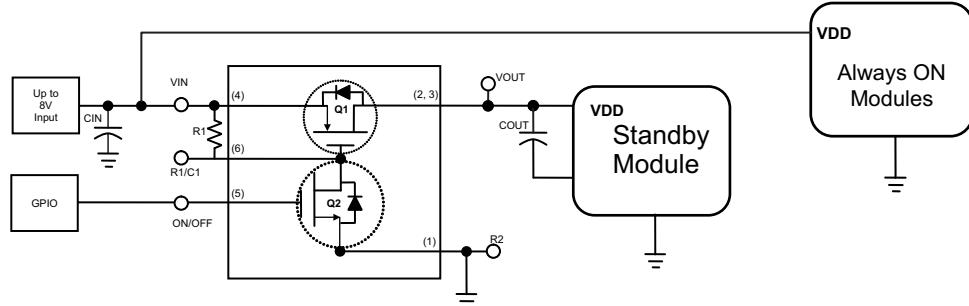
**Figure 5. Standby Power Generation Using TPS27081A**
