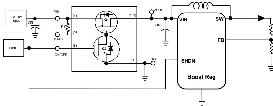
**Figure 6. True Shutdown Using TPS27081A**
