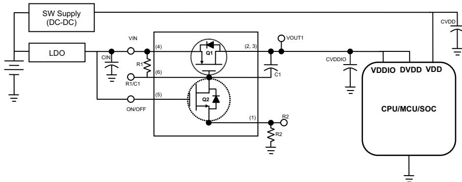
**Figure 7. Power Sequencing Using TPS27081A, Example 1**
