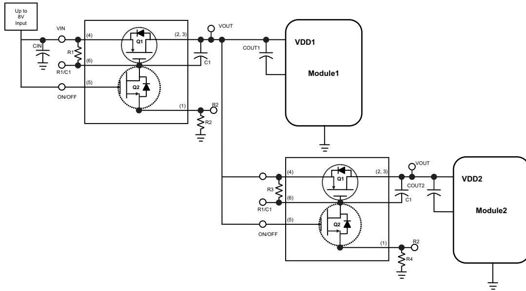
**Figure 9. Power Sequencing using TPS27081A, Example 3**
