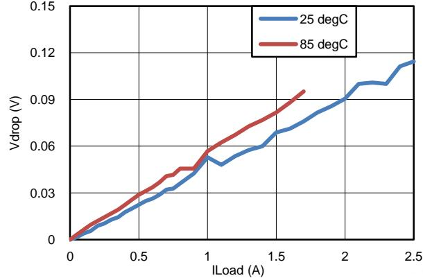
Figure 13. Vdrop vs IL;  $V_{GSQ1} = -3.3V$
