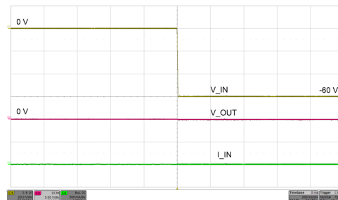
Figure 36. Reverse Input Supply Protection at -60 V
