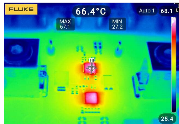
图 9-14. One (1) TPS25990 eFuse and one (1) TPS25985x eFuse in Parallel: Temperature Rise with 110-A DC Current at Room Temperature (No Air-Flow)
