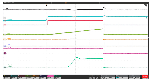
图 9-7. Power Up into Short: V_{IN} = 12 V, EN/UVLO Stepped Up From 0 V to 3 V, R_{IREF} = 40.2 k \Omega , R_{ILIM} on Each Device = 300 \Omega , and OUT Shorted to GND
