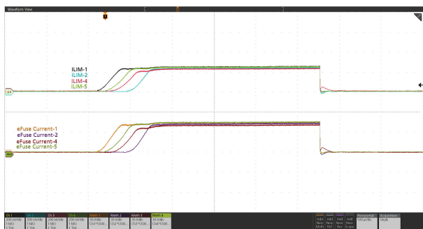
图 9-8. Power Up into Short (Current distribution among five devices in parallel): V_{IN} = 12 V, EN/UVLO Stepped Up From 0 V to 3 V, R_{IREF} = 40.2 k \Omega , R_{ILIM} on Each Device = 300 \Omega , and OUT Shorted to GND
