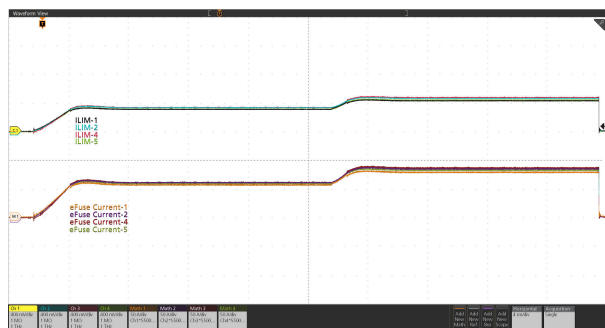
图 9-12. Circuit-Breaker Response (Current distribution among five devices in parallel): V_{IN} = 12\text{ V} , C_{ITIMER} = 22\text{ nF} , C_{LOAD} = 55\text{ mF} , R_{IMON} = 167\text{ }\Omega , R_{REF} = 40.2\text{ k}\Omega , and Load Current Stepped up From 300 A to 475 A for > 20 ms
