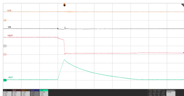
图 6-43. Circuit-Breaker Response TPS25974x
