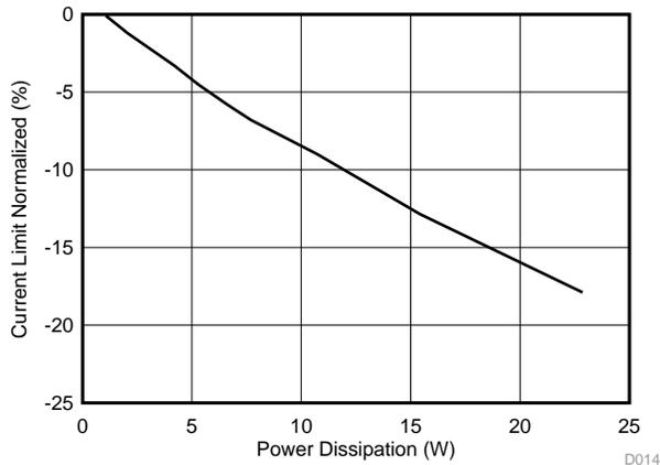
$$P_D = [V_{(IN)} - V_{(OUT)}] \cdot I_{LIMIT}$$
