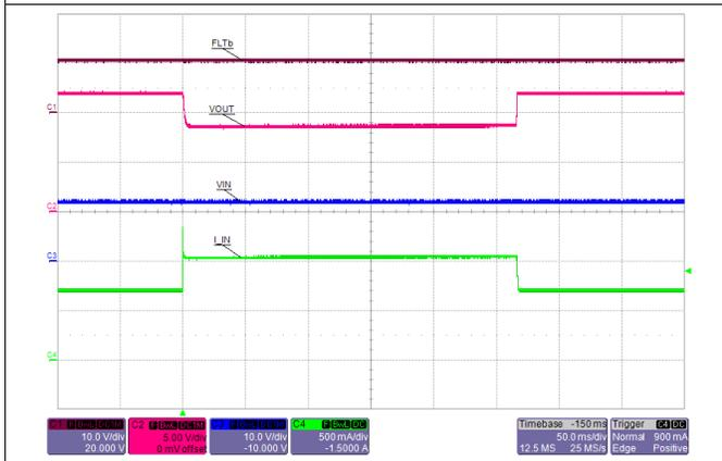
Figure 40. Over Load: Step Change in Load from 19 Ω to 9 Ω Back
