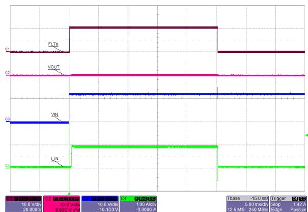
Figure 45. Hot Plug-in with Short on Output: Latched - TPS25921L
