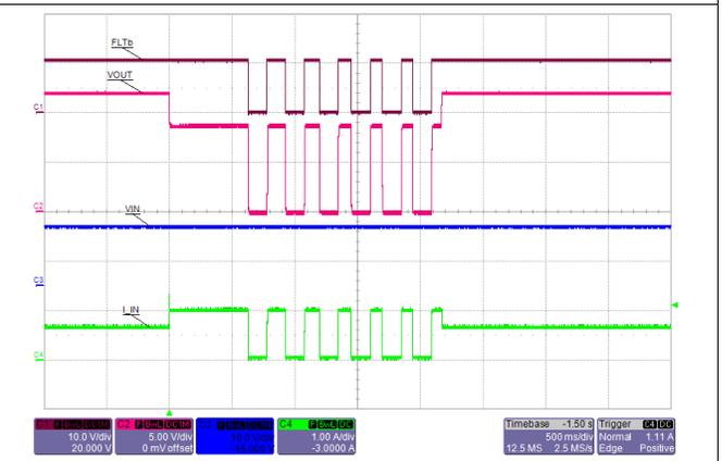
Figure 41. Overload Condition: Auto Retry and Recovery - TPS25921A
