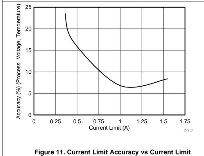
Figure 11. Current Limit Accuracy vs Current Limit
