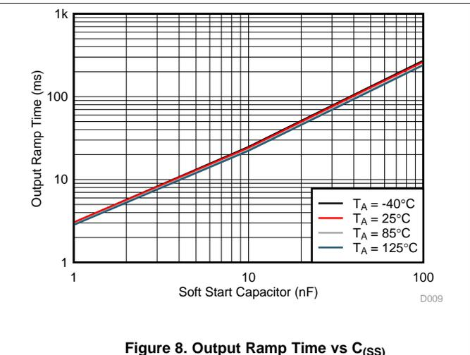
Figure 8. Output Ramp Time vs C<sub>(SS)</sub>
