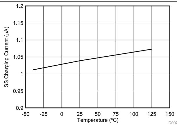
Figure 6. SS Pin Charging Current vs Temperature
