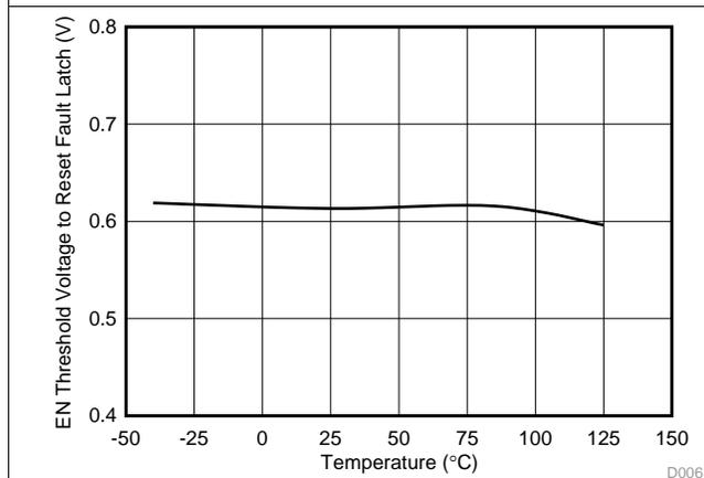
Figure 5. EN Threshold Voltage to Reset Fault Latch vs Temperature
