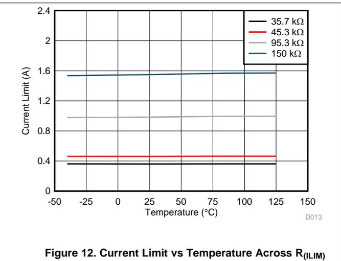
Figure 12. Current Limit vs Temperature Across R<sub>(ILIM)</sub>
