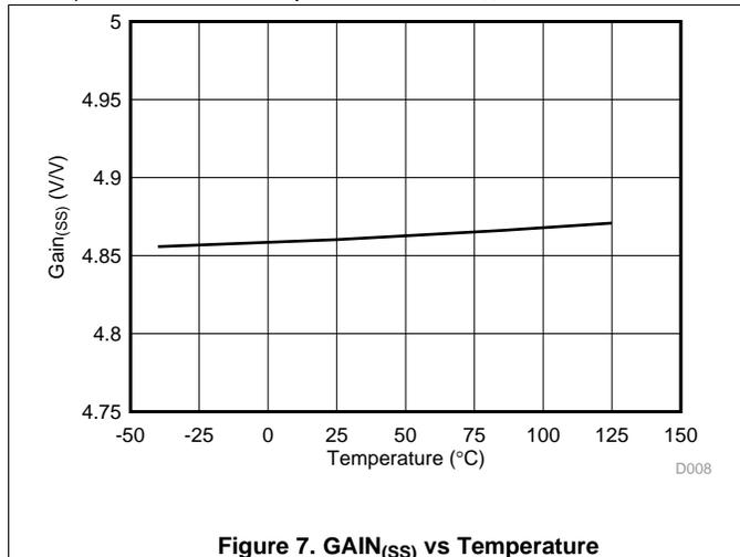
Figure 7. GAIN<sub>(SS)</sub> vs Temperature
