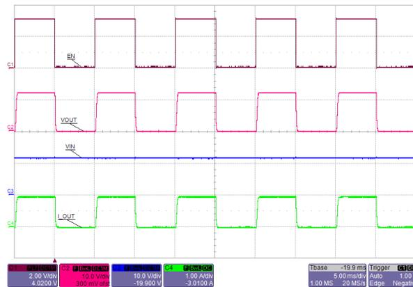
Figure 50. Smart Load Switch (100 Hz Operation)
