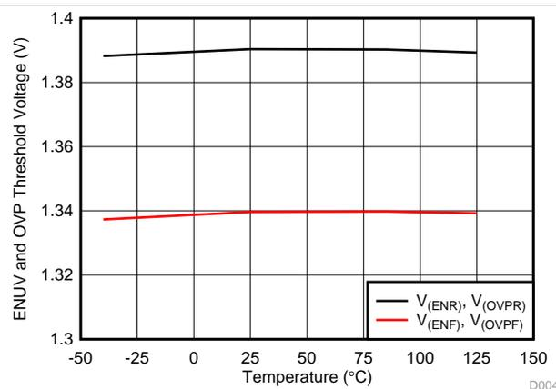
Figure 4. ENUV and OVP Threshold Voltage vs Temperature
