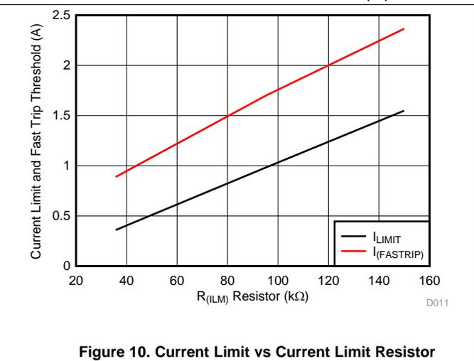
Figure 10. Current Limit vs Current Limit Resistor
