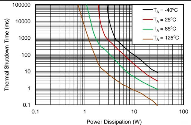
Taken on 1-Layer board, 2oz.(0.08-mm thick) with GND plane area: 14 cm<sup>2</sup> (bottom)
