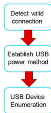
图 10-19. Flow of DFP-to-UFP Configuration
