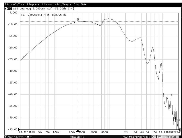
图 8-24. Off-state Data-Switch Isolation vs Frequency
