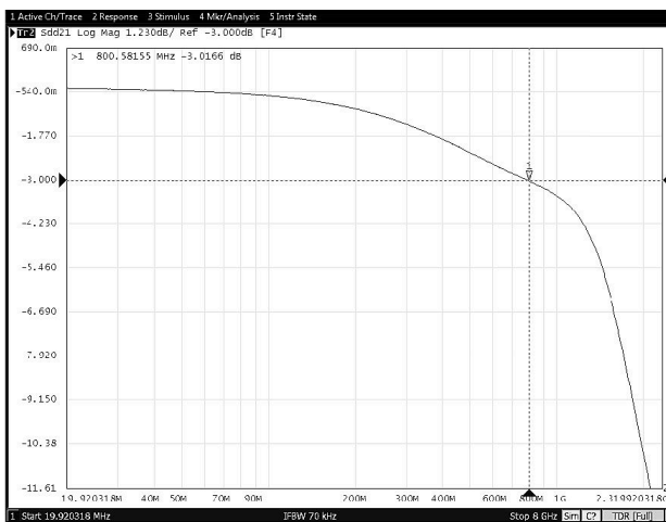
图 8-29. Data Transmission Characteristics vs Frequency (TPS25830A-Q1)
