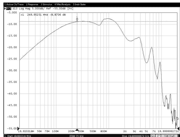
图 8-30. Off-State Data-Switch Isolation vs Frequency (TPS25830A-Q1)
