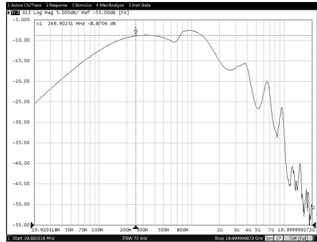
图 8-32. Off-State Data-Switch Isolation vs Frequency (TPS25830-Q1)
