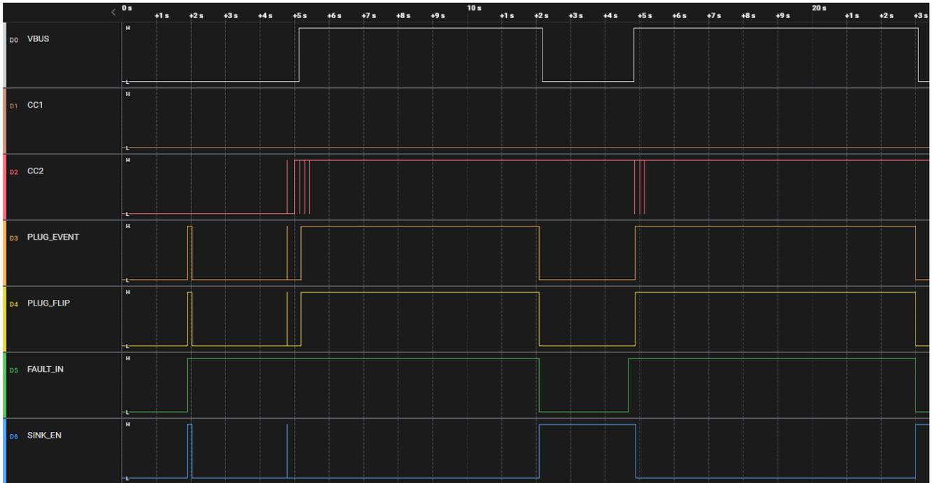
图 9-9. PLUG\_EVENT, PLUG\_FLIP,  $\overline{\text{FAULT\_IN}}$ , and  $\overline{\text{SINK\_EN}}$  -  $\overline{\text{FAULT\_IN}}$  Input
