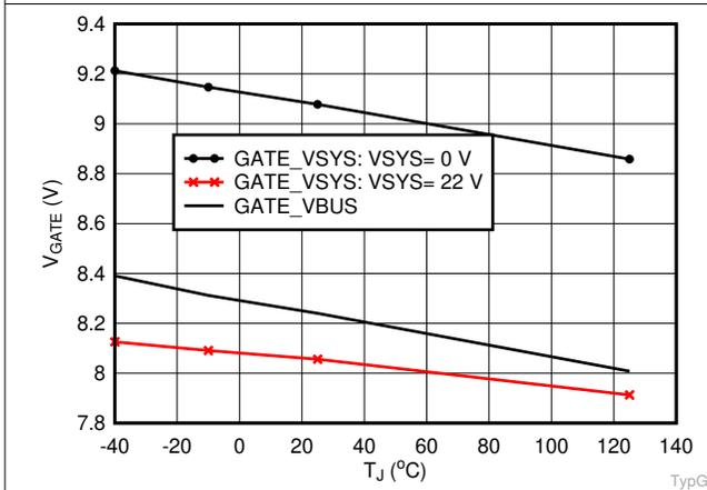
图 6-5. V<sub>GATE\_VBUS\_ON</sub> vs. Temperature for TPS25730S
