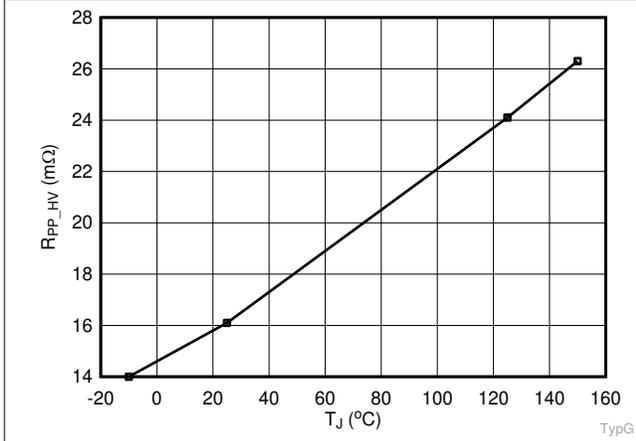
图 6-3. R<sub>PPHV</sub> vs. Temperature for TPS25730D
