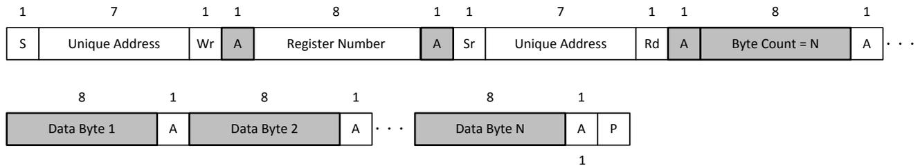
图 8-24. I<sup>2</sup>C Unique Address Read Register Protocol
