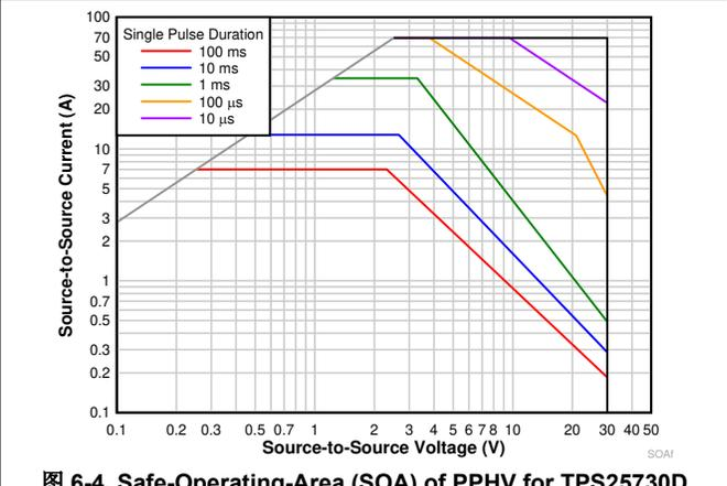
图 6-4. Safe-Operating-Area (SOA) of PPHV for TPS25730D
