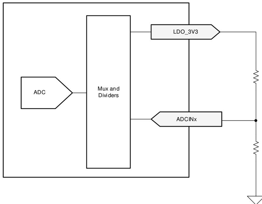
图 8-17. ADCINx Resistor Divider
