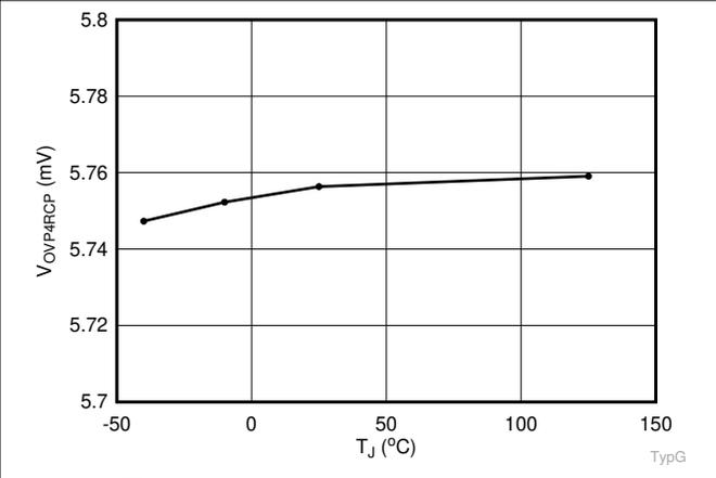
图 6-2. V<sub>OVP4RCP</sub> (Setting 2) vs. Temperature
