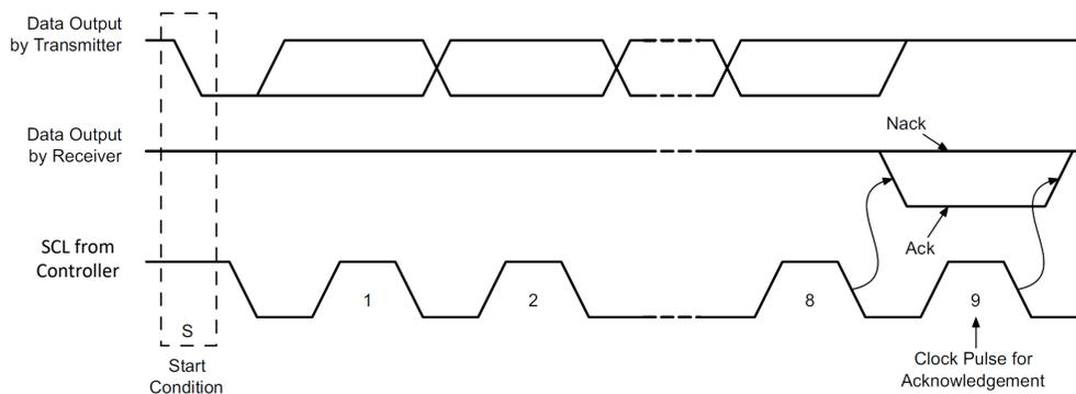
图 8-22. I<sup>2</sup>C Acknowledgment
