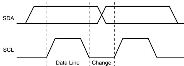
图 8-21. I<sup>2</sup>C Bit Transfer
