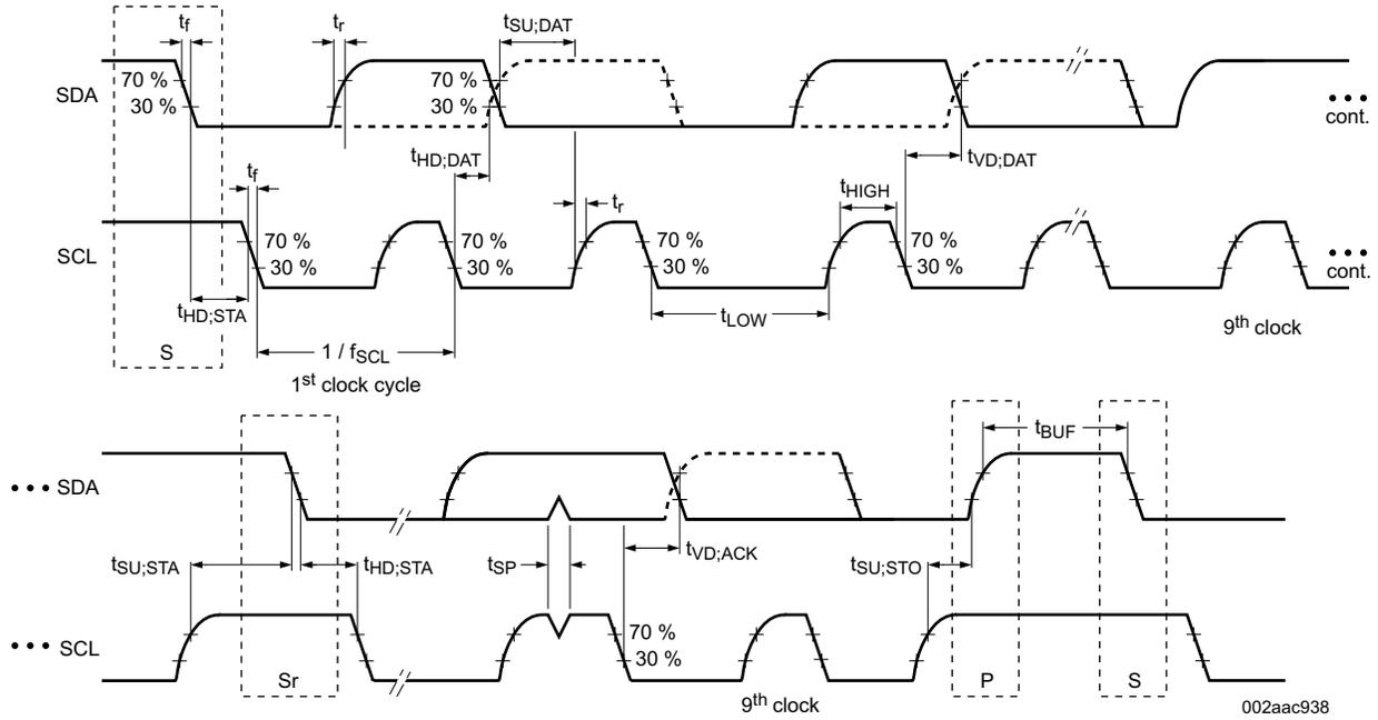
图 7-1. I<sup>2</sup>C Target Interface Timing
