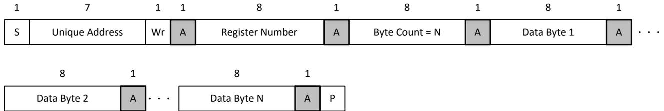
图 8-23. I<sup>2</sup>C Unique Address Write Register Protocol
