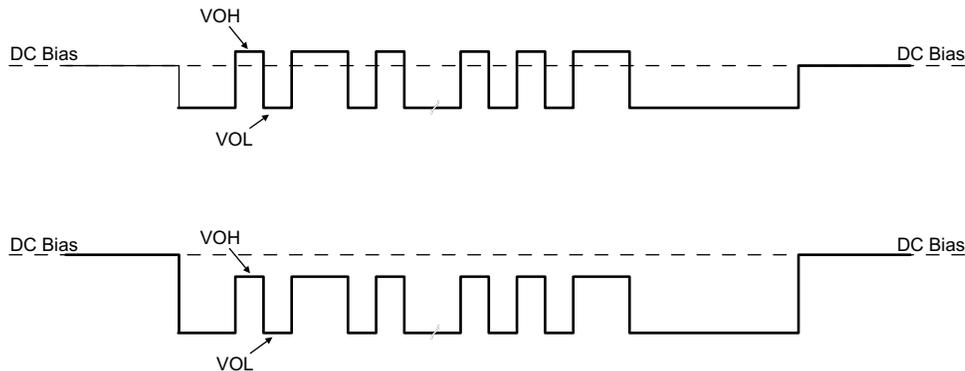
图 8-8. TX Driver Transmission with DC Bias
