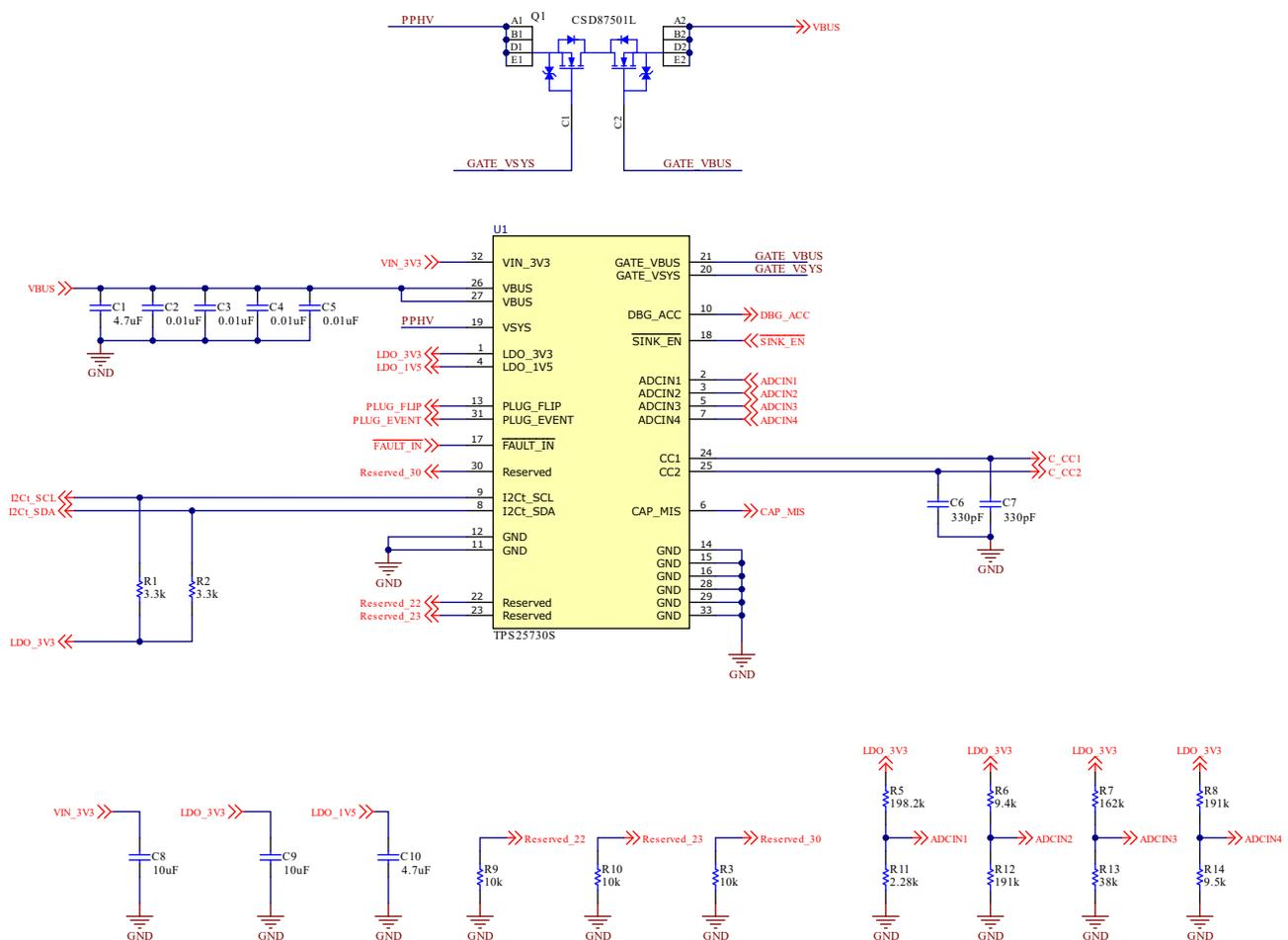
图 9-20. Example Schematic
