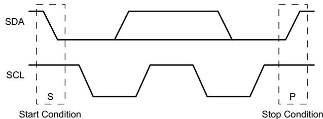
图 8-20. I<sup>2</sup>C Definition of Start and Stop Conditions
