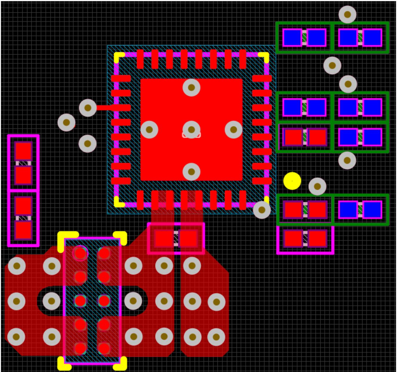
图 9-26. VBUS Copper Pours and Via Placement
