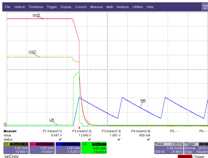
Figure 34. TPS2483 Retry-Cycle Timing Detail
