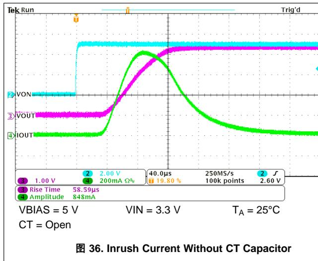
图 36. Inrush Current Without CT Capacitor
