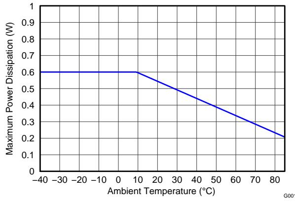
**Figure 8. Allowable Power Dissipation**
