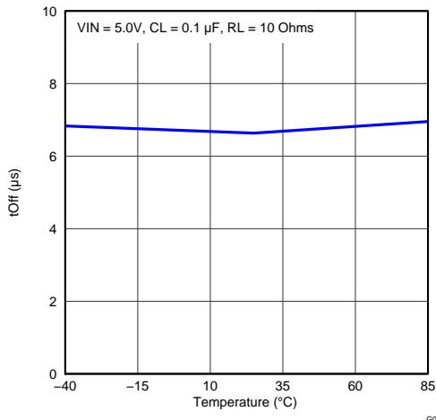
**Figure 43. Turn-Off Time vs Temperature**
