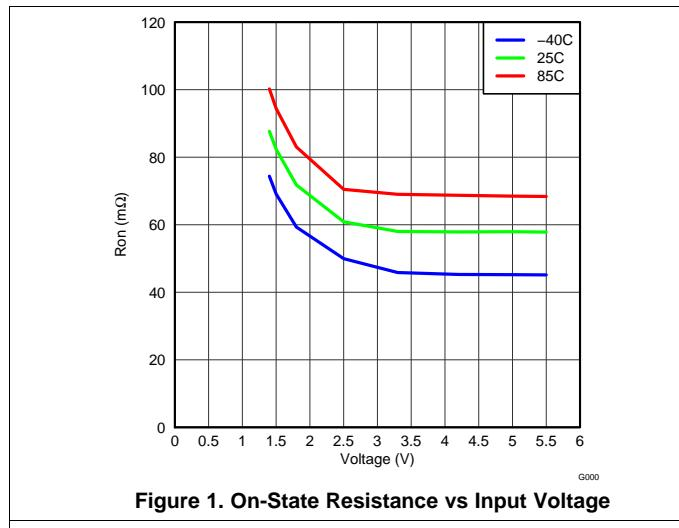
Figure 1. On-State Resistance vs Input Voltage
