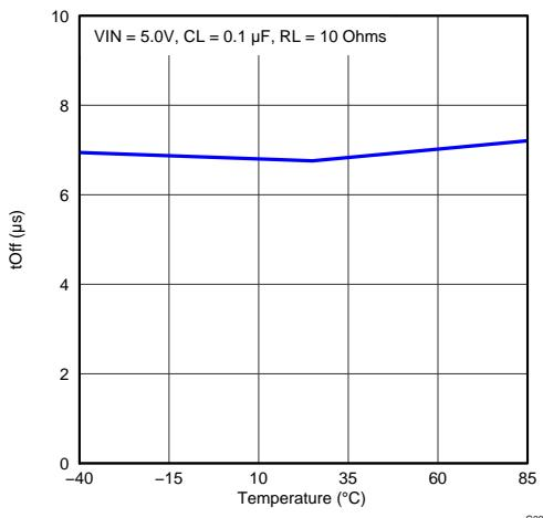
**Figure 25. Turn-off Time vs Temperature**
