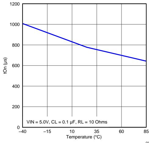
**Figure 42. Turn-on Time vs Temperature**
