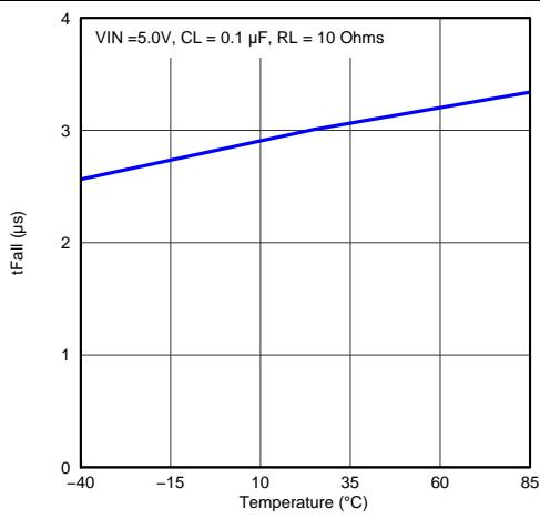
**Figure 39. Fall Time vs Temperature**
