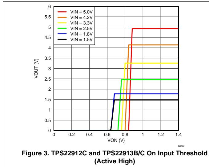
Figure 3. TPS22912C and TPS22913B/C On Input Threshold (Active High)
