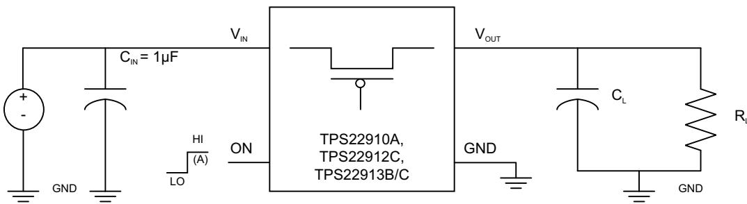
**Figure 47. Timing Test Circuit**
