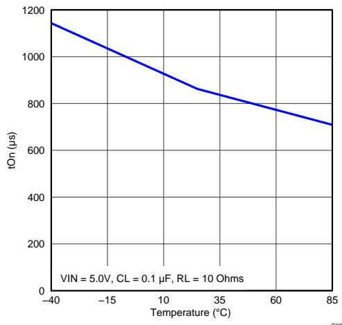
**Figure 24. Turn-on Time vs Temperature**
