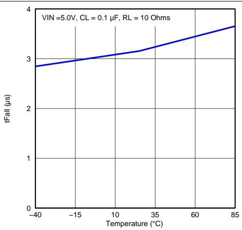
**Figure 21. Fall Time vs Temperature**
