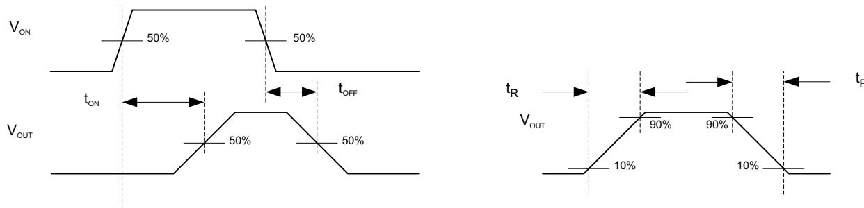
A. Rise and fall times of the control signal is 100 ns.
