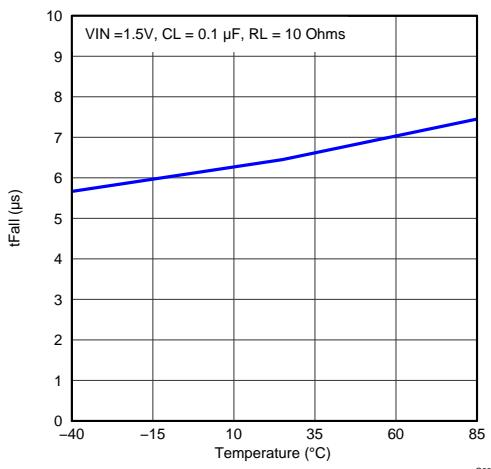
**Figure 23. Fall Time vs Temperature**
