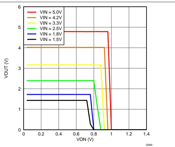
Figure 2. TPS22910A On Input Threshold (Active Low)
