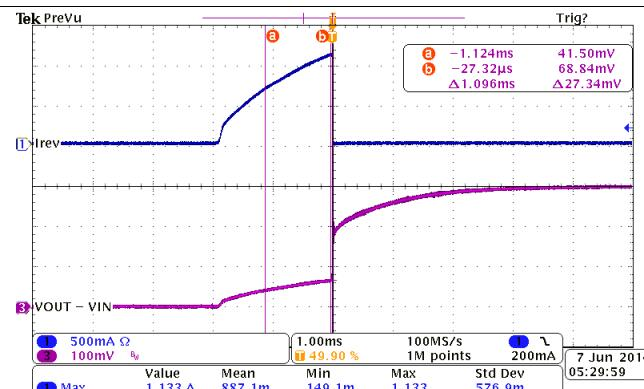
**Figure 10. Full-Time Reverse Current Protection**
