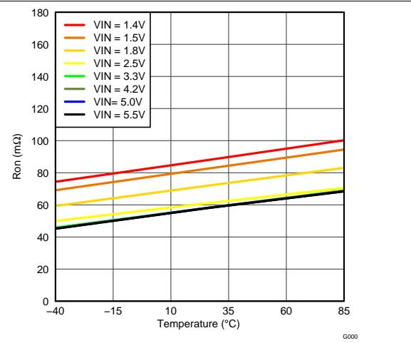
Figure 6. On-state Resistance vs Temperature
