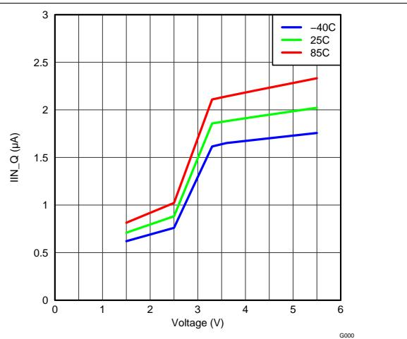
Figure 4. Input Current, Quiescent vs Input Voltage
