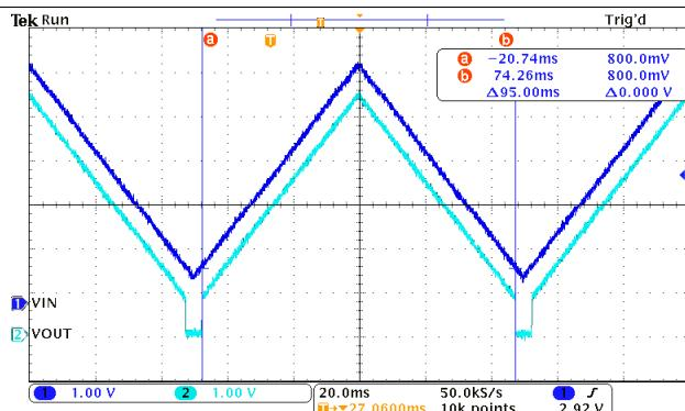
**Figure 9. Under Voltage Lockout Response**
