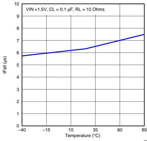
**Figure 41. Fall Time vs Temperature**
