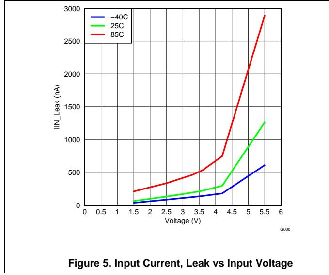
Figure 5. Input Current, Leak vs Input Voltage
