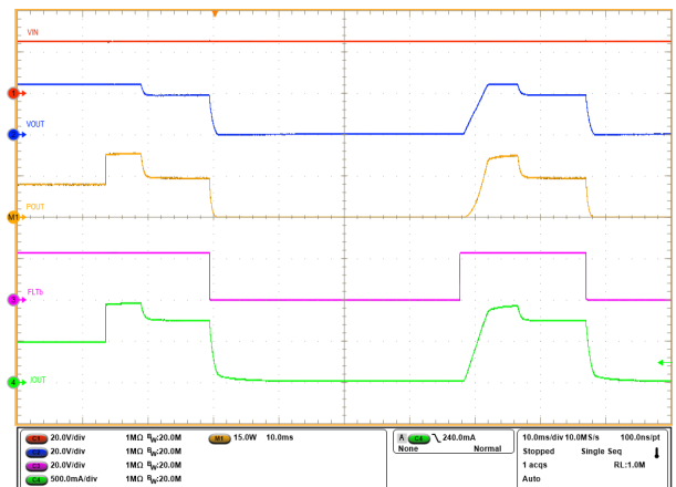
图 9-5. 15-W Power Limiting with TPS16410 ( I_{OUT} < I_{ocp} )
