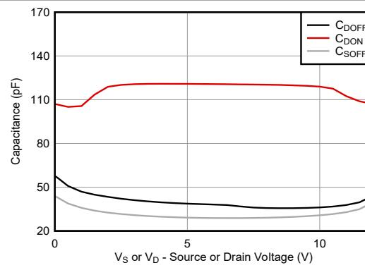
图 5-28. Capacitance vs Source Voltage or Drain Voltage
