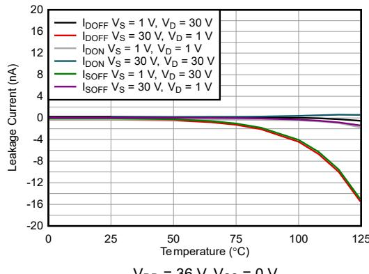
图 5-11. Leakage Current vs Temperature
