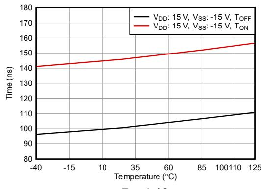
图 5-18. T<sub>ON</sub> and T<sub>OFF</sub> vs Temperature
