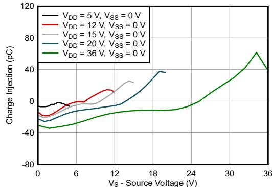
图 5-16. Charge Injection vs Source Voltage - Single Supplies
