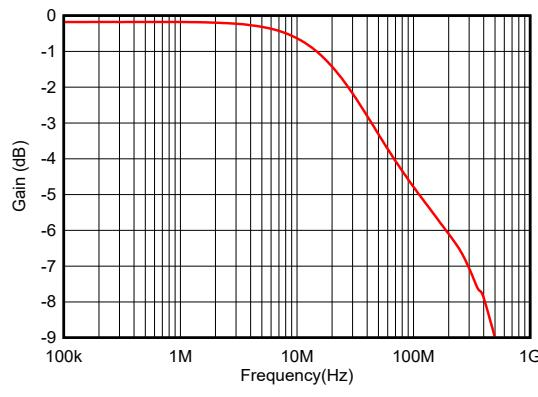
图 5-25. On Response vs Frequency
