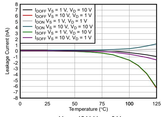
图 5-12. Leakage Current vs Temperature
