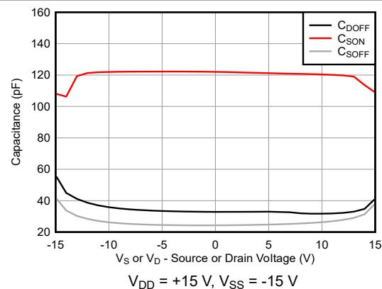
图 5-27. Capacitance vs Source Voltage or Drain Voltage
