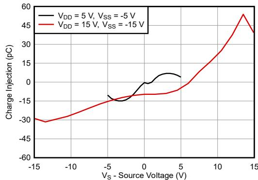
图 5-14. Charge Injection vs Source Voltage - Dual Supplies
