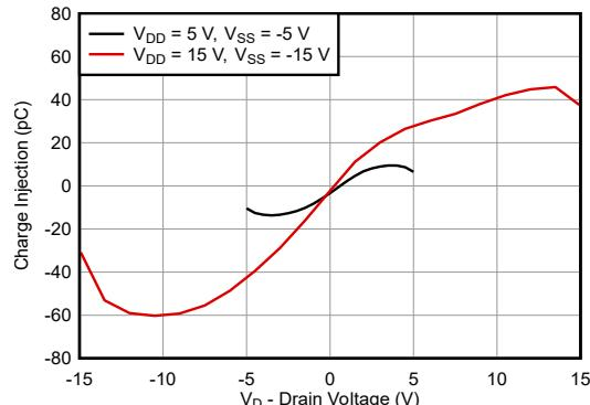
图 5-15. Charge Injection vs Drain Voltage - Dual Supplies
