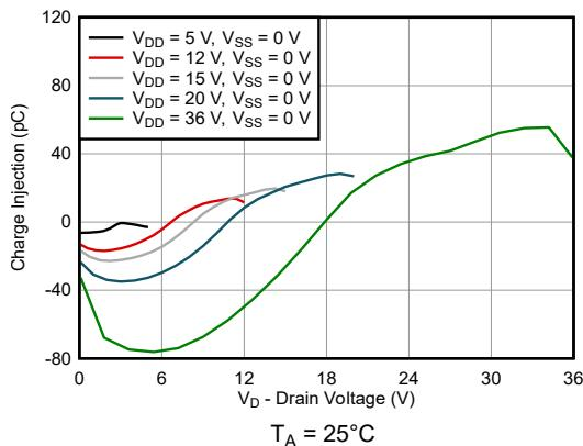
图 5-17. Charge Injection vs Drain Voltage - Single Supplies
