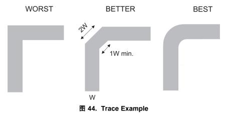
Route the high-speed signals using a minimum of vias and corners which reduces signal reflections and impedance changes. When a via must be used, increase the clearance size around it to minimize its capacitance. Each via introduces discontinuities in the signal's transmission line and increases the chance of picking up interference from the other layers of the board. Be careful when designing test points, through-hole pins are not recommended at high frequencies.
