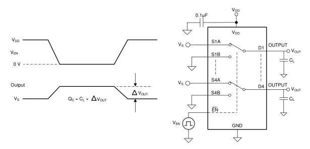
图 37. Charge-Injection Measurement Setup
