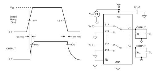
图 33. t<sub>ON (VDD)</sub> and t<sub>OFF (VDD)</sub>Time Measurement Setup
