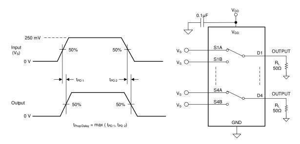
图 35. Propagation Delay Measurement Setup
