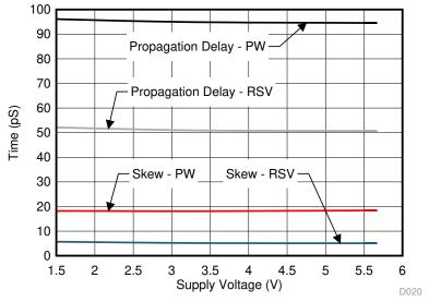
图 43. Propagation Delay and Skew Measurement
