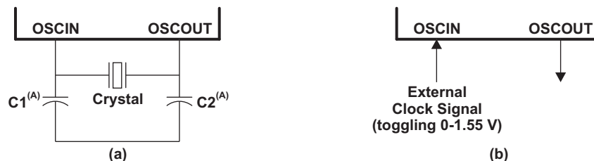
Figure 5-3. Recommended Crystal/Clock Connection
