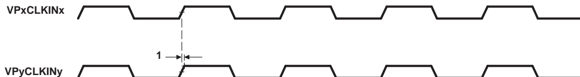
Figure 5-57. Video Port Dual-Display Sync Timing
