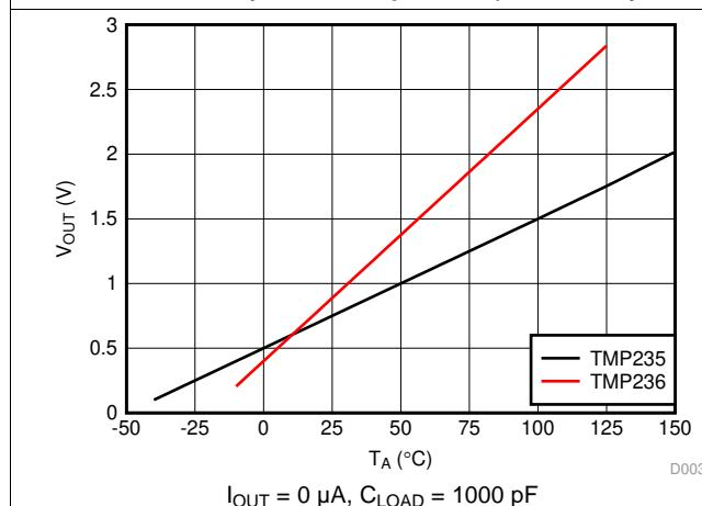
图 3. Output Voltage vs. Ambient Temperature
