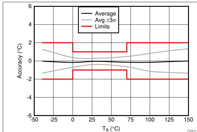
图 1. Accuracy vs.  $T_A$  Temperature (A2 Accuracy Level)
