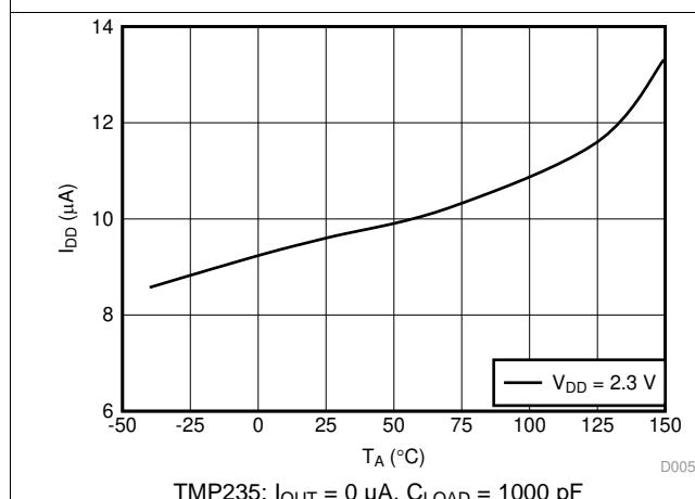
图 5. Supply Current vs. Temperature
