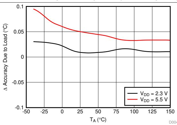
图 4. Changes in Accuracy vs. Ambient Temperature (Due to Load)
