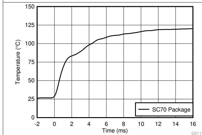
TMP235: 1 x 1 (inches) PCB, Air 26°C to Fluid Bath 123°C
