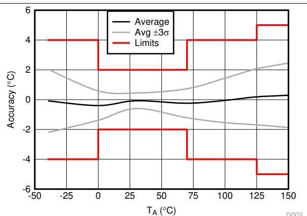
图 2. Accuracy vs.  $T_A$  Temperature (A4 Accuracy Level)
