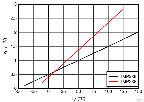
Figure 14. Output Voltage vs. Ambient
