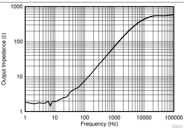
TMP235:  $T_A = 25^\circ\text{C}$ ,  $V_{DD} = 5$  V,  $I_{OUT} = 100$   $\mu\text{A}$
