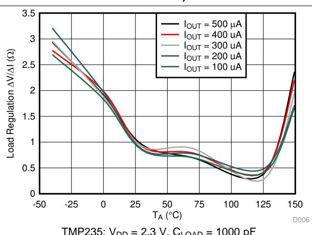
图 6. Load Regulation vs. Ambient Temperature
