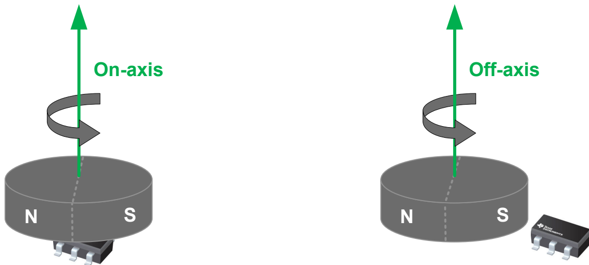
图 8-11. On-Axis vs Off-Axis Angle Measurements
