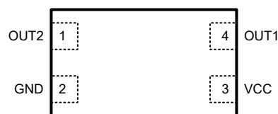
Figure 5-2. ZFC Package, 4-Pin X1LGA (Top View)
