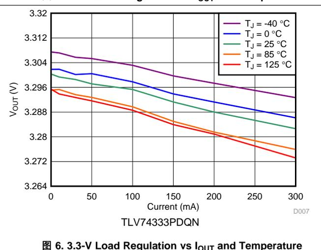
图 6. 3.3-V Load Regulation vs  $I_{OUT}$  and Temperature
