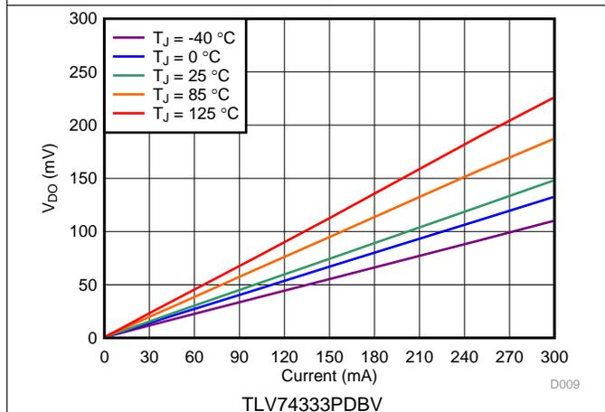
图 11. 3.3-V Dropout Voltage vs  $I_{OUT}$  and Temperature
