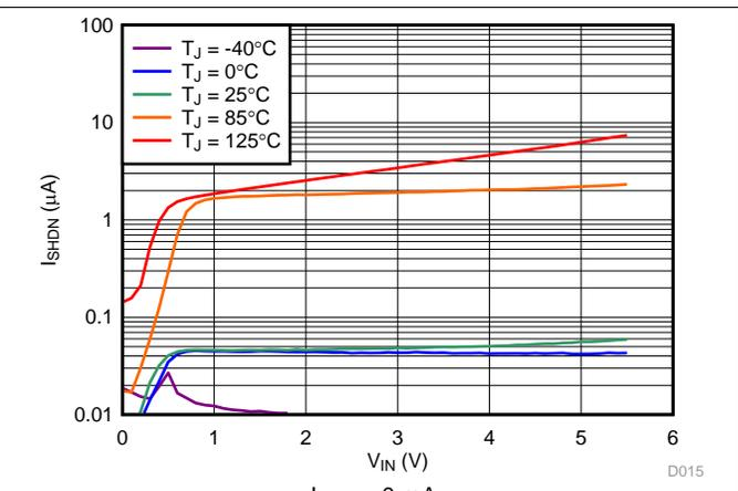
图 16. Shutdown Current vs  $V_{IN}$  and Temperature
