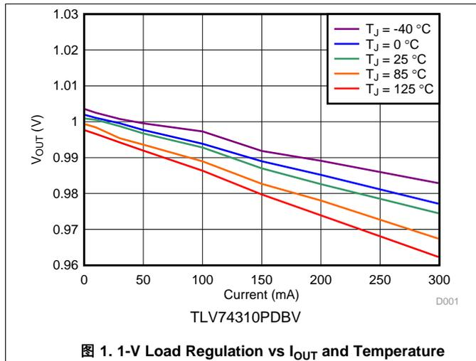
图 1. 1-V Load Regulation vs  $I_{OUT}$  and Temperature
