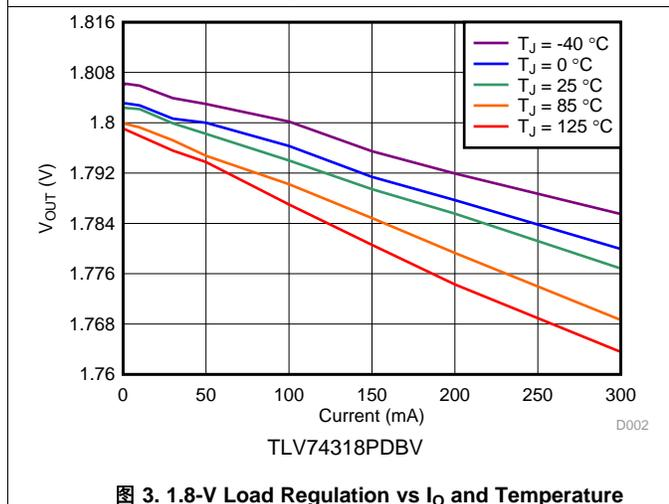
图 3. 1.8-V Load Regulation vs  $I_O$  and Temperature
