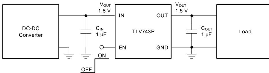
图 32. DC/DC Converter Post Regulation
