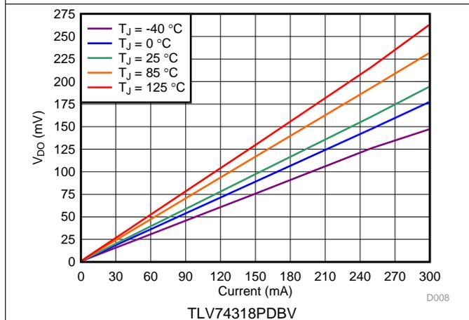
图 9. 1.8-V Dropout Voltage vs  $I_{OUT}$  and Temperature
