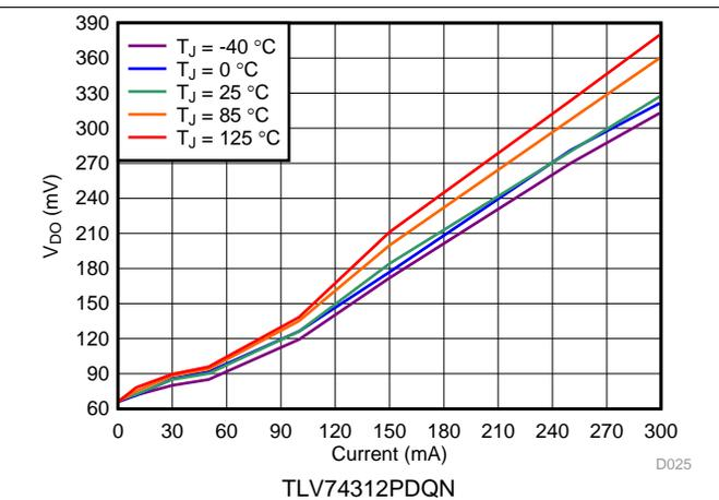
图 8. 1.2-V Dropout Voltage vs  $I_{OUT}$  and Temperature
