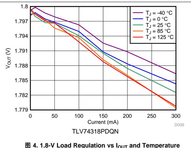
图 4. 1.8-V Load Regulation vs  $I_{OUT}$  and Temperature
