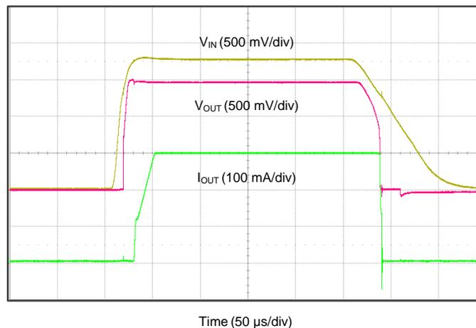
图 33. 1.8-V to 1.5-V Regulation at 300 mA
