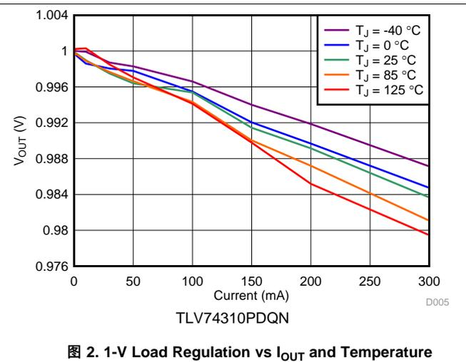
图 2. 1-V Load Regulation vs  $I_{OUT}$  and Temperature
