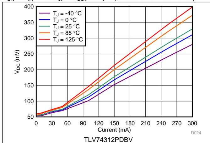
图 7. 1.2-V Dropout Voltage vs  $I_{OUT}$  and Temperature
