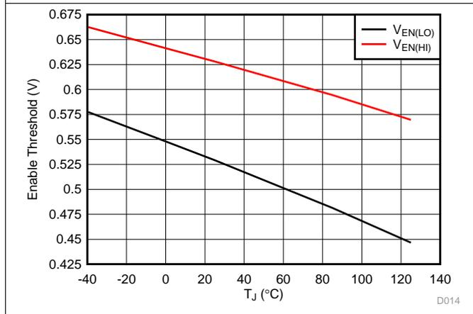
图 17. Enable Threshold vs Temperature
