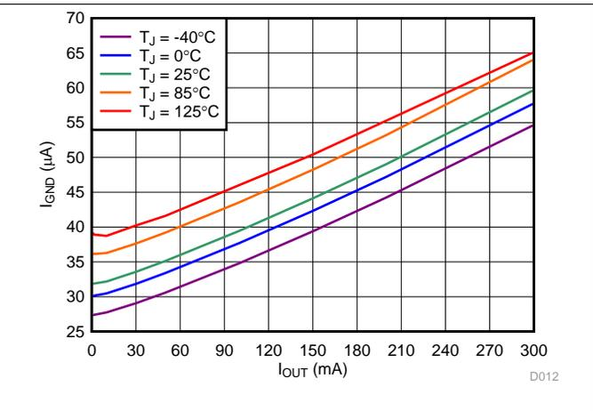
图 14. Ground Pin Current vs  $I_{OUT}$  and Temperature
