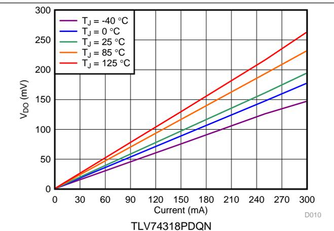
图 10. 1.8-V Dropout Voltage vs  $I_{OUT}$  and Temperature
