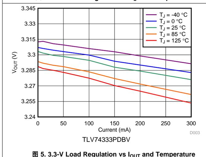
图 5. 3.3-V Load Regulation vs  $I_{OUT}$  and Temperature
