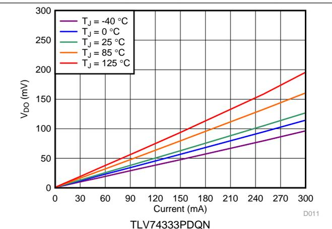
图 12. 3.3-V Dropout Voltage vs  $I_{OUT}$  and Temperature
