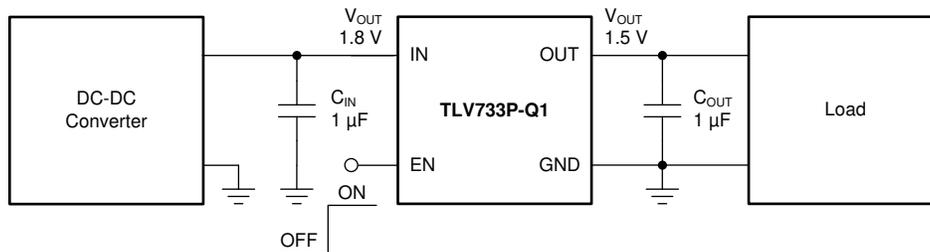
图 8-2. DC-DC Converter Post Regulation
