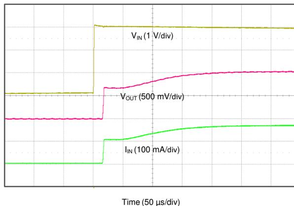
图 8-5. No Inrush Startup, 3.0-V to 1.0-V Regulation
