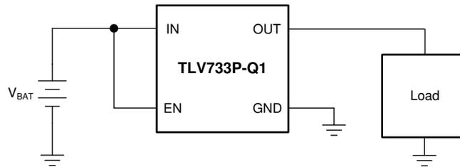
图 8-4. Capacitor-Free Operation from a Battery Input Supply
