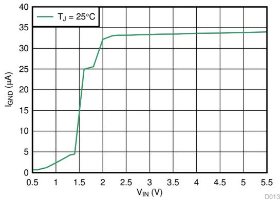
**图 6-3. Ground Pin Current vs  $V_{IN}$**
