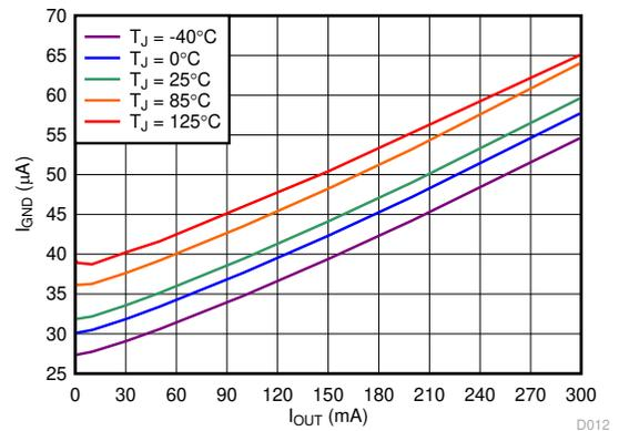
**图 6-2. Ground Pin Current vs  $I_{OUT}$  and Temperature**
