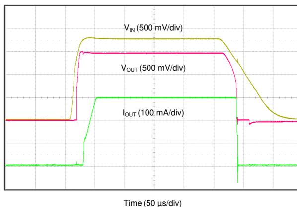
图 8-3. 1.8-V to 1.5-V Regulation at 300 mA
