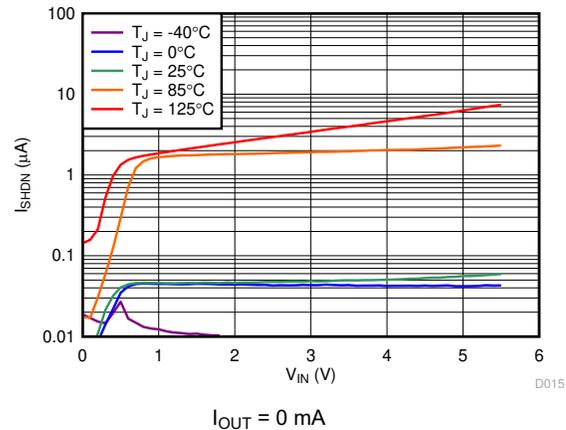
**图 6-4. Shutdown Current vs  $V_{IN}$  and Temperature**
