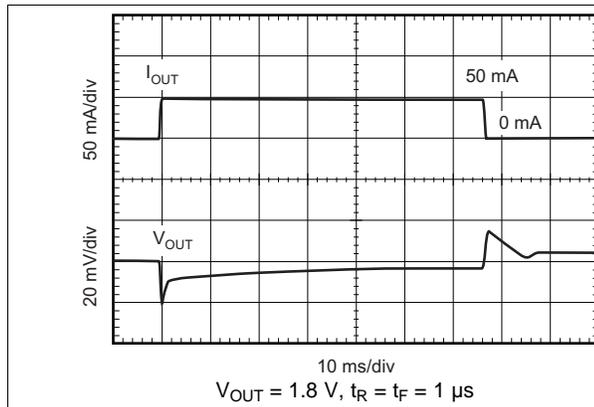
**Figure 23. Load Transient Response**
