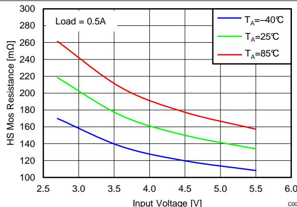
**图 7. High-Side FET  $R_{DS(on)}$  vs Input Voltage**
