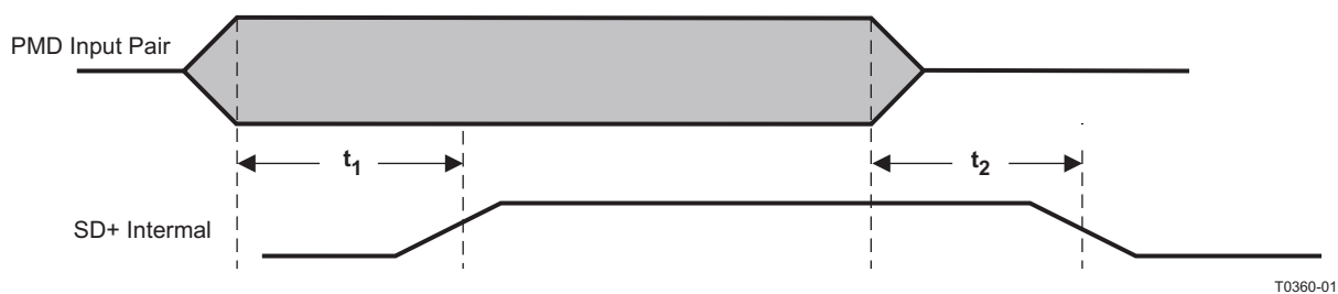
Figure 9-20. 100Base-TX Signal Detect Timing
