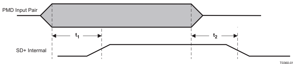
Figure 9-20. 100Base-TX Signal Detect Timing
