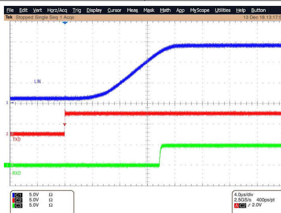
图 10-13. Dominant to Recessive Propagation Delay
