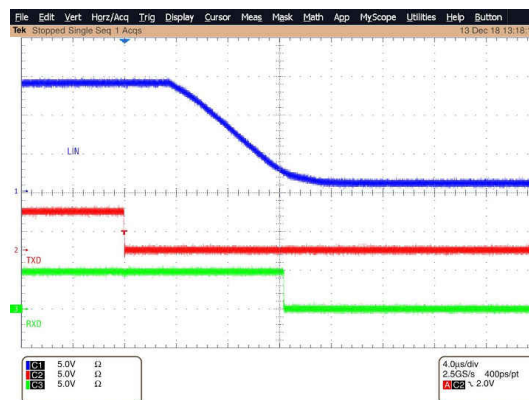
图 9-12. Recessive to Dominant Propagation Delay
