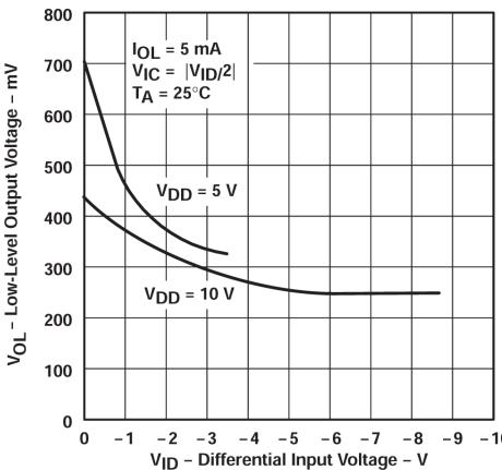
Figure 5-11. Low-level Output Voltage vs Differential Input Voltage
