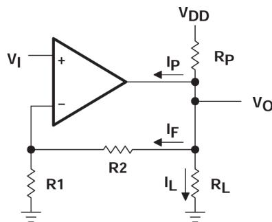
$$R_P = \frac{V_{DD} - V_O}{I_F + I_L + I_P}$$
