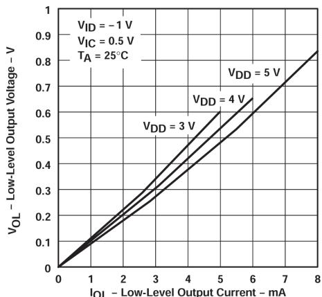
Figure 5-13. Low-level Output Voltage vs Low-level Output Current
