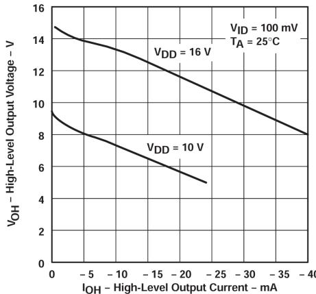
Figure 5-6. High-level Output Voltage vs High-level Output Current
