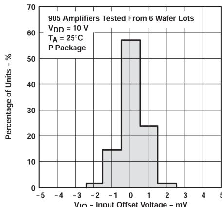
Figure 5-2. Distribution of TLC27L2 Input Offset Voltage
