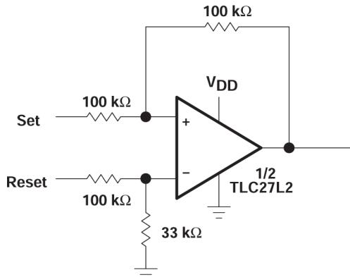
Figure 7-10. Set/Reset Flip-Flop,  $V_{DD} = 5\text{V}$  to  $12\text{V}$
