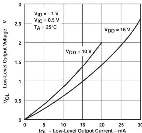
Figure 5-14. Low-level Output Voltage vs Low-level Output Current
