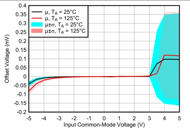
**Figure 7-4. Offset Voltage vs Input Common-mode Voltage**
