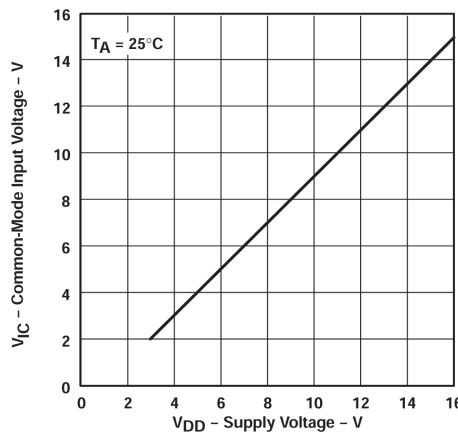
Figure 5-18. Common-mode Input Voltage Positive Limit vs Supply Voltage
