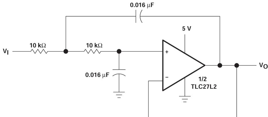
**Figure 7-13. Two-Pole Low-Pass Butterworth Filter,  $V_{DD} = 5\text{V}$  to  $16\text{V}$**
