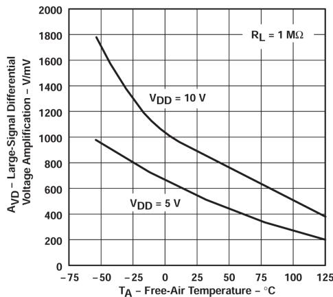
Figure 5-16. Large-signal Differential Voltage Amplification vs Free-air Temperature
