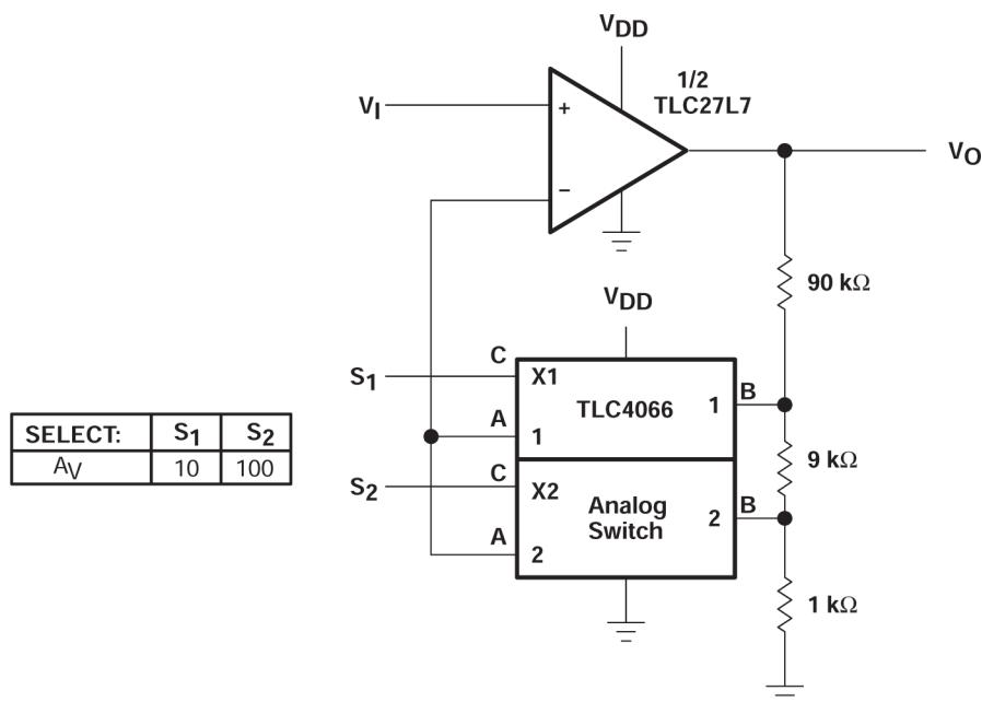
Figure 7-11. Amplifier with Digital Gain Selection,  $V_{DD} = 5\text{V}$  to  $16\text{V}$
