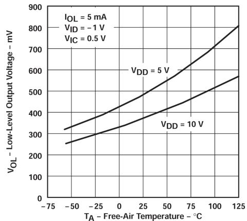
Figure 5-12. Low-level Output Voltage vs Free-air Temperature
