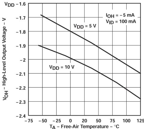
Figure 5-8. High-level Output Voltage vs Free-air Temperature
