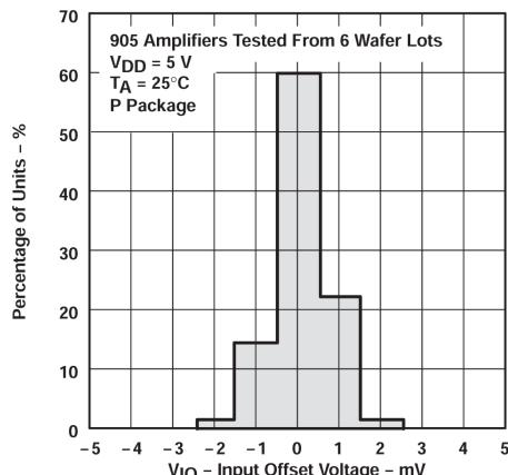
Figure 5-1. Distribution of TLC27L2 Input Offset Voltage
