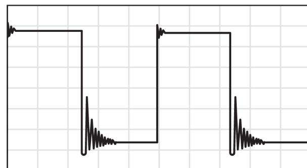
(b)  $C_L = 260 \text{ pF}, R_L = \text{NO LOAD}$
