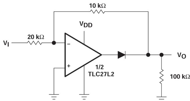
Figure 7-12. Full-Wave Rectifier, Normalized to  $f_c = 1\text{kHz}$  and  $R_L = 10\text{k}\Omega$
