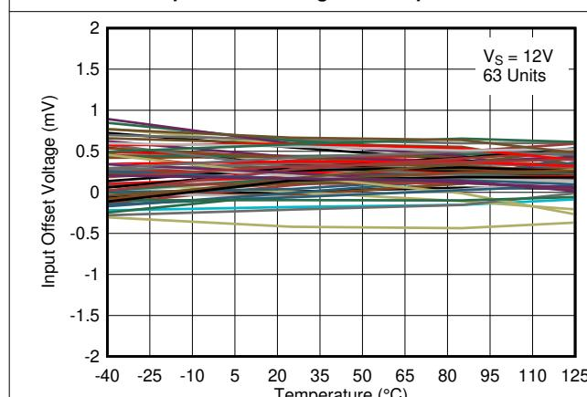
图 5-17. Input Offset Voltage vs. Temperature at 12V
