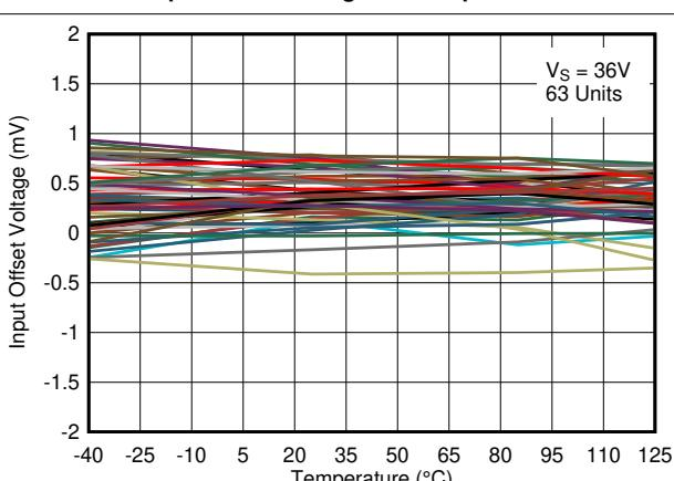
图 5-18. Input Offset Voltage vs. Temperature at 36V
