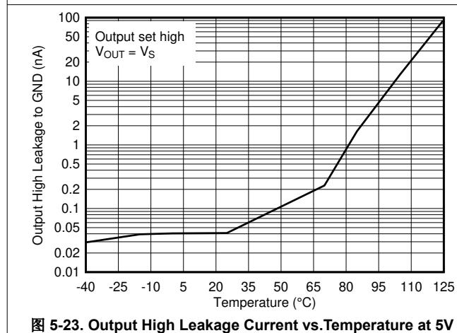
图 5-23. Output High Leakage Current vs. Temperature at 5V
