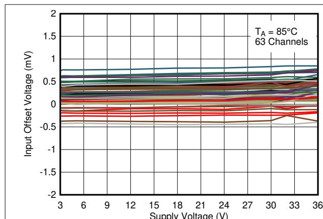
图 5-13. Input Offset Voltage vs. Supply Voltage at  $85^\circ\text{C}$
