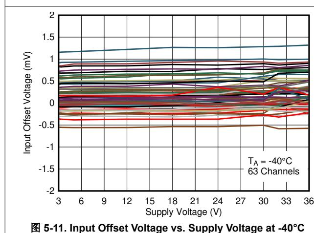
图 5-11. Input Offset Voltage vs. Supply Voltage at -40°C
