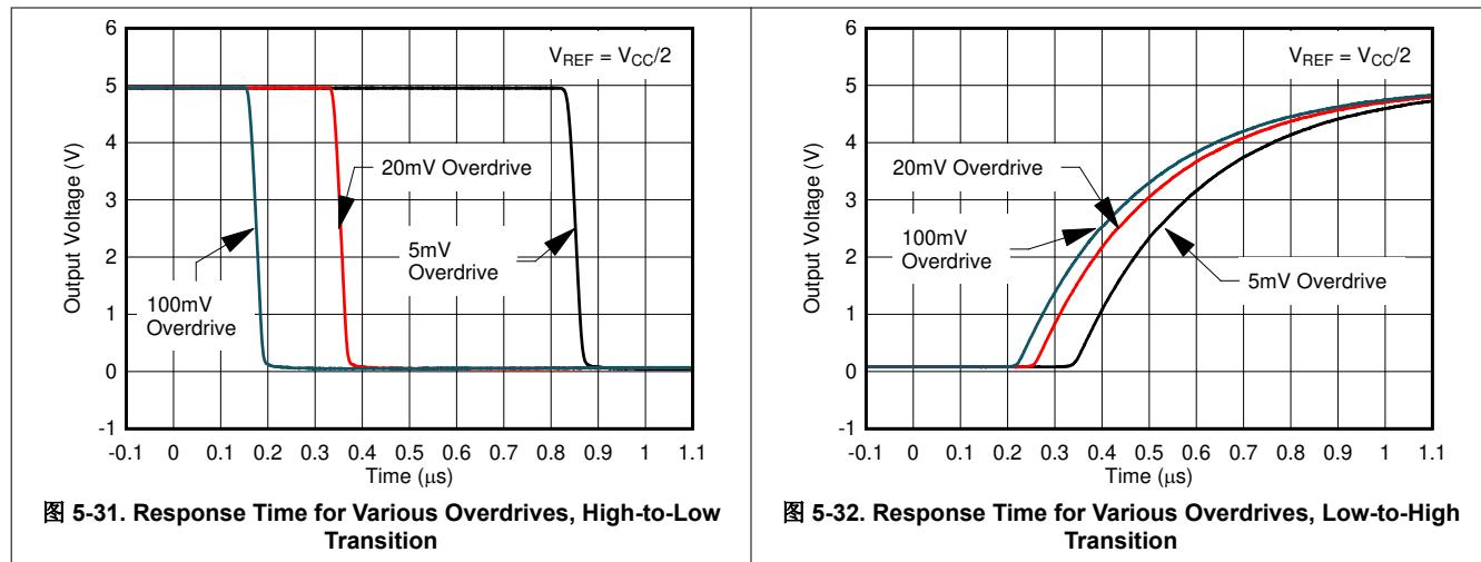
图 5-31. Response Time for Various Overdrives, High-to-Low Transition
