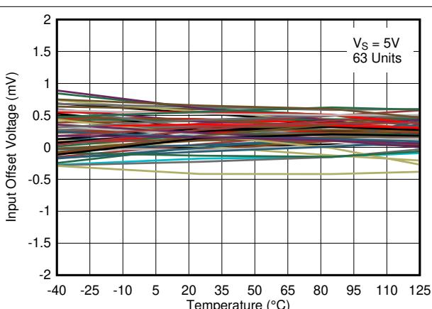
图 5-16. Input Offset Voltage vs. Temperature at 5V
