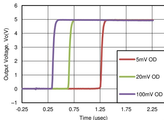
图 7-2. Response Time for Various Overdrives (Positive Transition)
