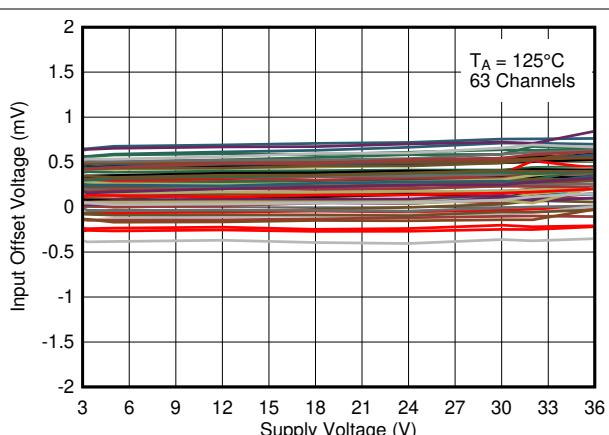
图 5-14. Input Offset Voltage vs. Supply Voltage at  $125^\circ\text{C}$
