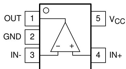
Note reversed inputs compared to similar common pinout
