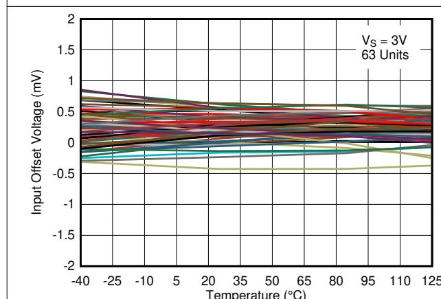
图 5-15. Input Offset Voltage vs. Temperature at 3V
