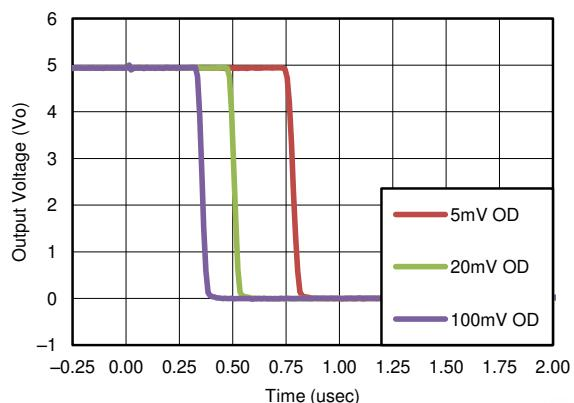
图 7-3. Response Time for Various Overdrives (Negative Transition)
