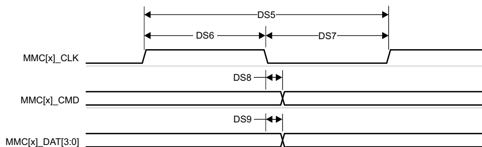
图 6-98. MMC1/2 – Default Speed – Transmit Mode
