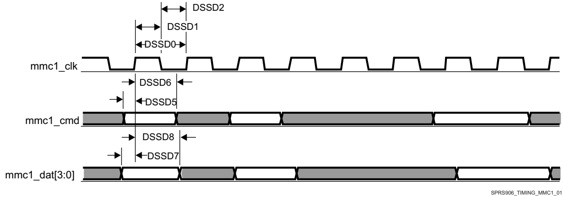
图 7-54. MMC/SD/SDIO in - Default Speed - Receiver Mode
