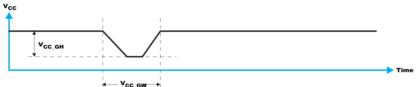
Figure 30. Glitch Width and Glitch Height
