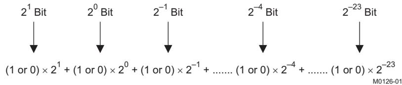
Figure 35. Conversion Weighting Factors—3.23 Format to Floating Point
