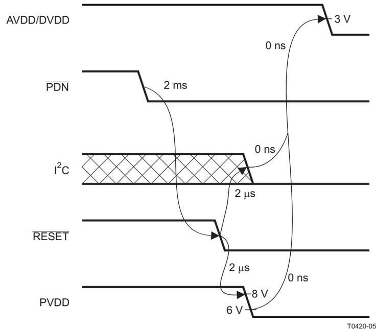
Figure 38. Power-Loss Sequence
