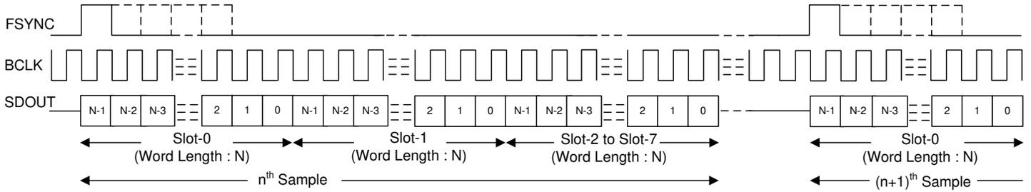
图 6-4. TDM 模式协议时序 (TX\_OFFSET = 0 且 BCLK\_POL = 1)
