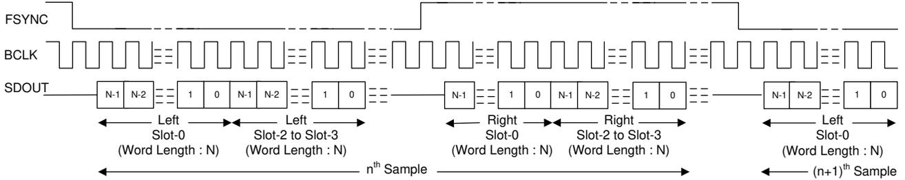
图 6-8. I<sup>2</sup>S 协议时序 (TX\_OFFSET = 0 且 BCLK\_POL = 1)
