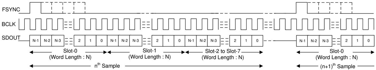
图 6-4. TDM 模式协议时序 (TX\_OFFSET = 0 且 BCLK\_POL = 1)
