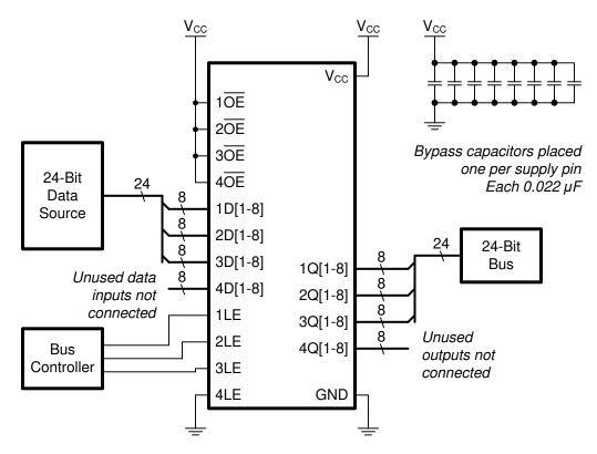
图 8-1. Simplified schematic for typical application
