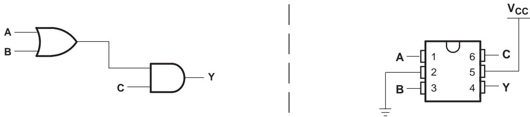
Figure 3. Y = (A + B) \bullet C
