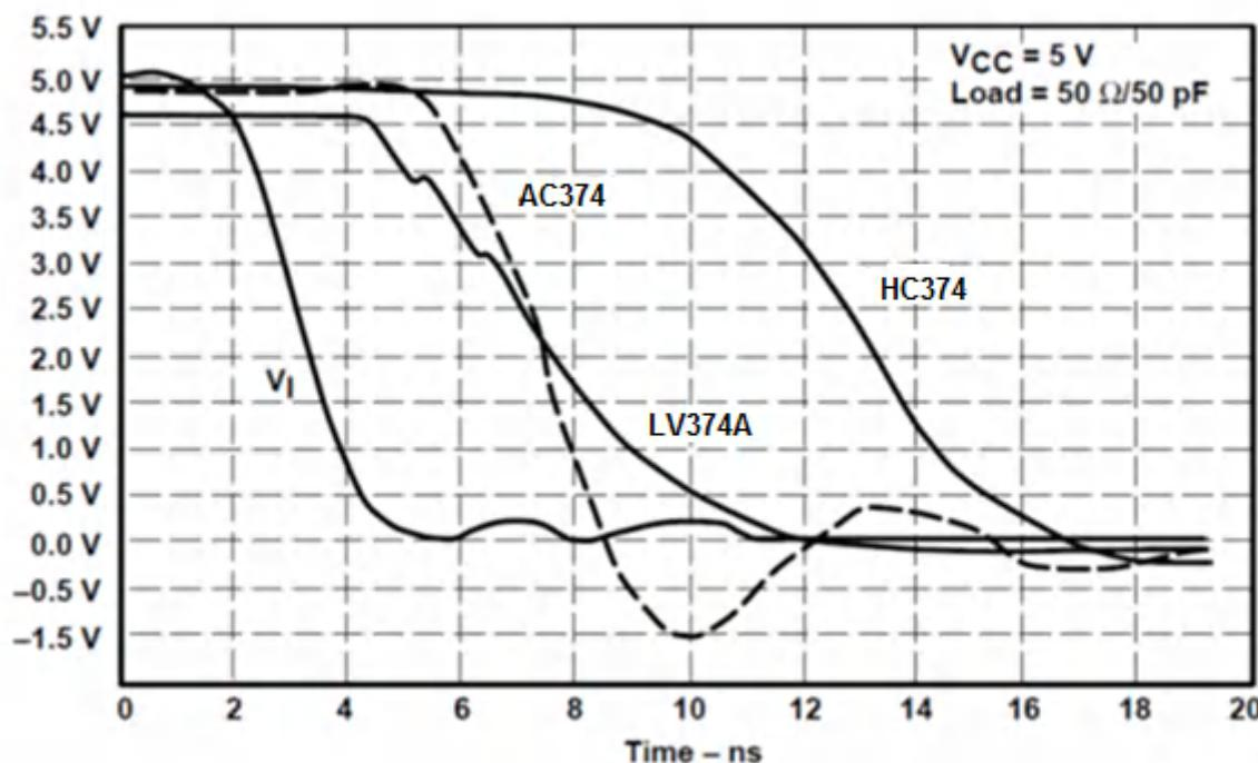
图 9-2. Switching Characteristics Comparison
