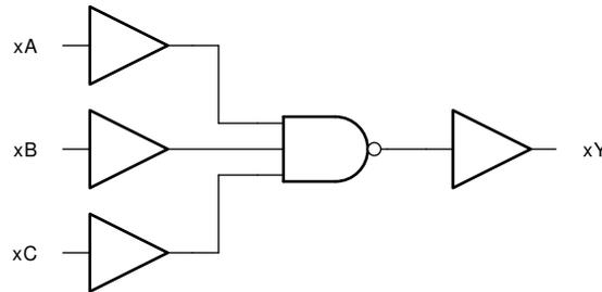
图 8-1. Simplified Schematic
