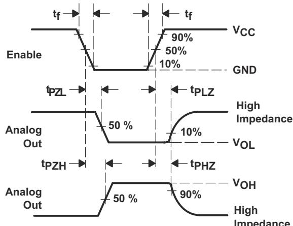
图 6-9. Propagation Delays, Enable to Analog Out
