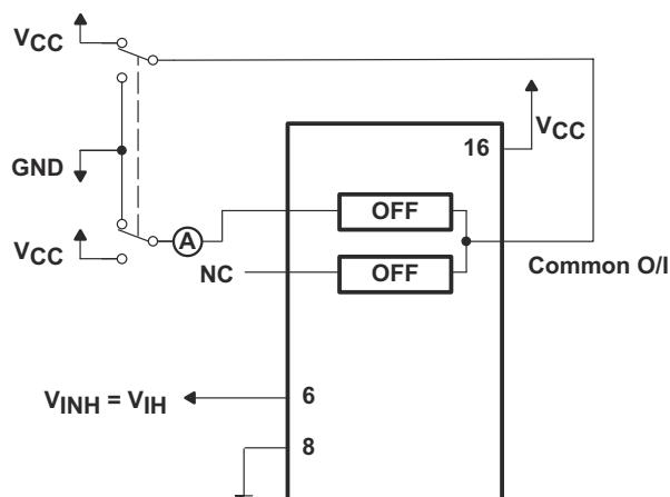
图 6-2. Maximum Off-Channel Leakage Current,
