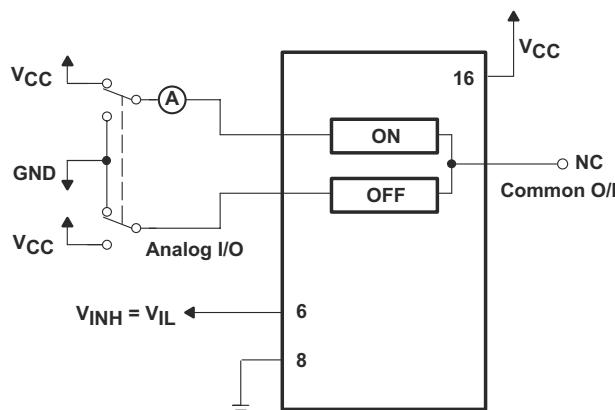
图 6-4. Maximum On-Channel Leakage Current,
