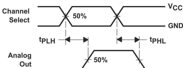
图 6-5. Propagation Delays, Channel Select to
