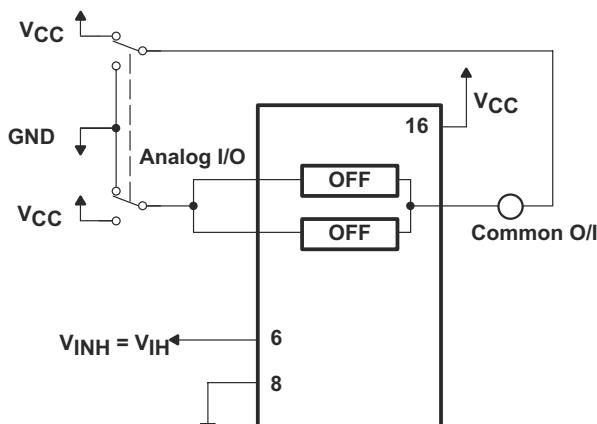
图 6-3. Maximum Off-Channel Leakage Current,
