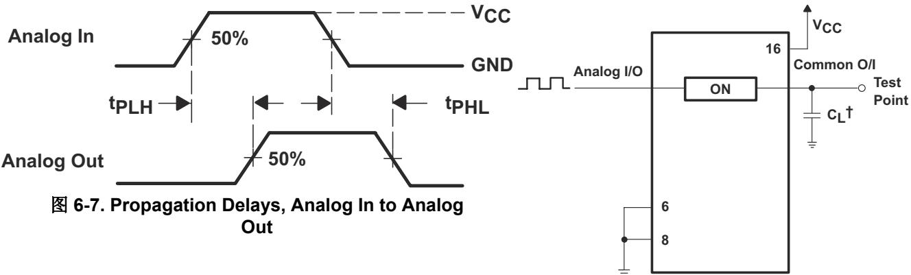
图 6-7. Propagation Delays, Analog In to Analog Out
