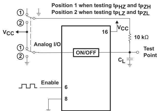
图 6-10. Propagation-Delay Test Setup, Enable to Analog Out
