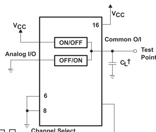
† Includes all probe and jig capacitance
