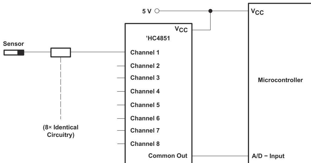
图 8-3. Solution by Applying the ' HC4851 Multiplexer
