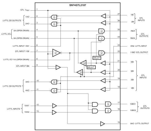
(1) The enable on 7BO1/7BO2 includes a delay that prevents a transient condition (where 5BI/6BI go from low to high, and the low to high on 5A/6A lags up to 100 ns) from causing a low glitch on the 7BO1/7BO2 outputs.
