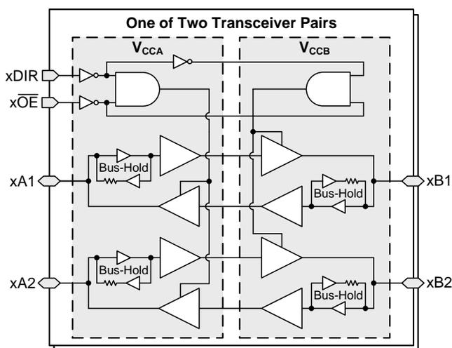
Note: Bus-hold circuits are only present for data inputs, not control inputs
