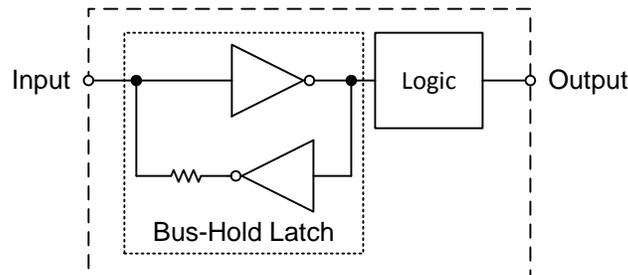
图 10. Simplified Schematic For Device With Bus-Hold Data Inputs
