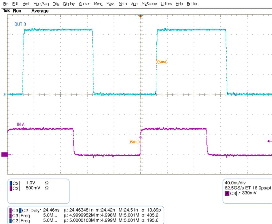
图 12. Up Translation at 2.5 MHz (0.7 V to 3.3 V)
