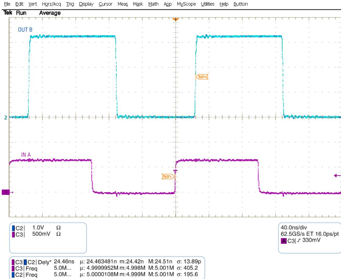
图 8-4. Up Translation at 2.5 MHz (0.7V to 3.3V)
