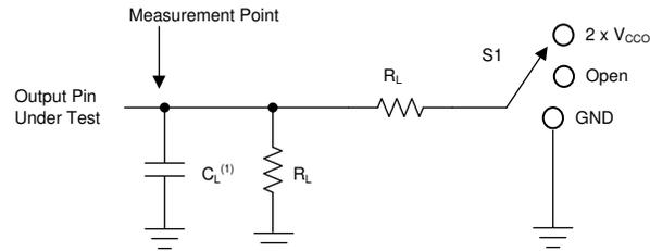
A.  $C_L$  includes probe and jig capacitance.
