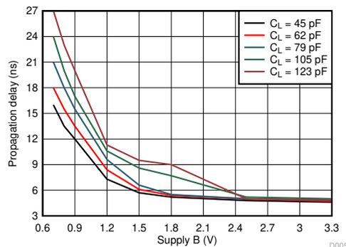
$T_A = 25^\circ\text{C}$   $V_{CCA} = 1.8\text{V}$
