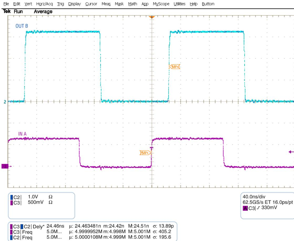
图 8-2. Up Translation at 2.5 MHz (0.7V to 3.3V)
