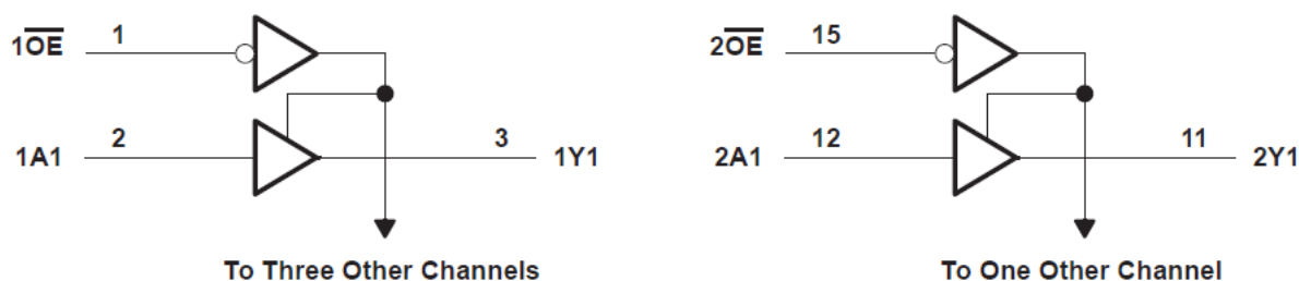
图 7-1. Logic Diagram (Positive Logic)
